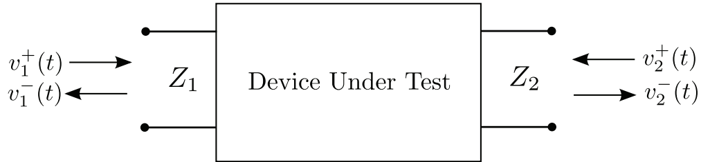
Figure 3.8: The two-port model of an electronic device. Input voltages are labeled with a subscript 1 and output voltages are labeled with a subscript 2. The input and output ports are ideal 50 \, \Omega transmission lines.
