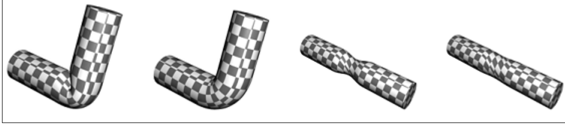
Figure 3.1: Skinning is subject to a variety of artifact. Common forms of deformation artifact occur when an object loses volume when bent, an effect known as “pinch” (a) or when an object is rotated, experiencing the “candy-wrapper effect” (b). (Images courtesy of Merry et al [69].)
