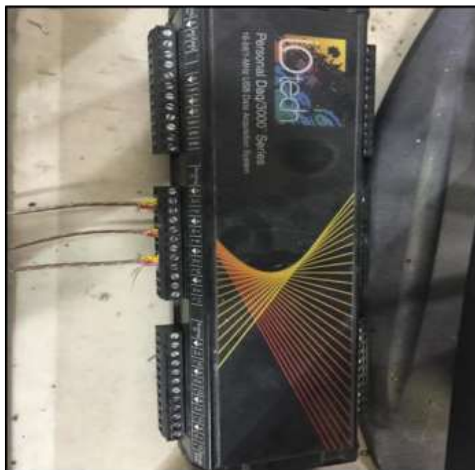
Figure 3.7: Temperature data acquisition device utilized as part of this study
