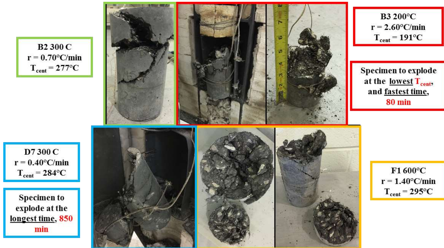
Figure 3.26: UHPC specimens following experiencing explosive spalling in electrical furnace
