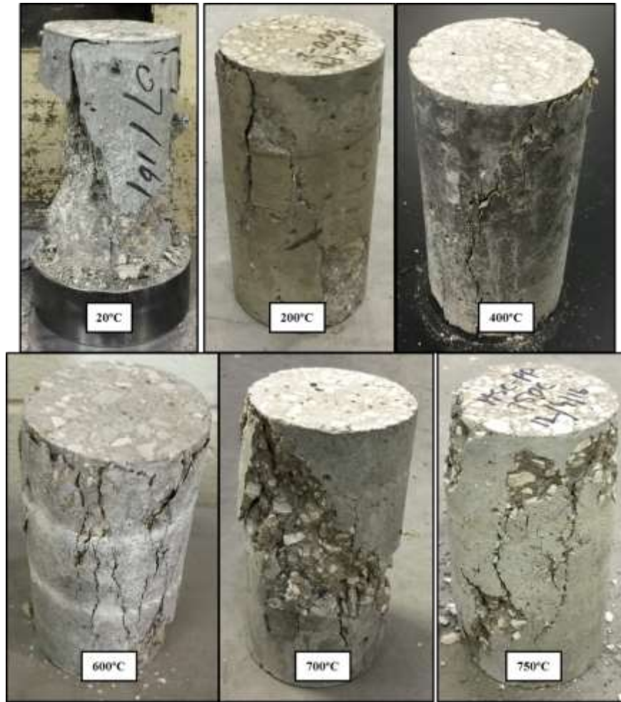
Figure 3.18: Failure modes of HSC – PP at respective temperatures
