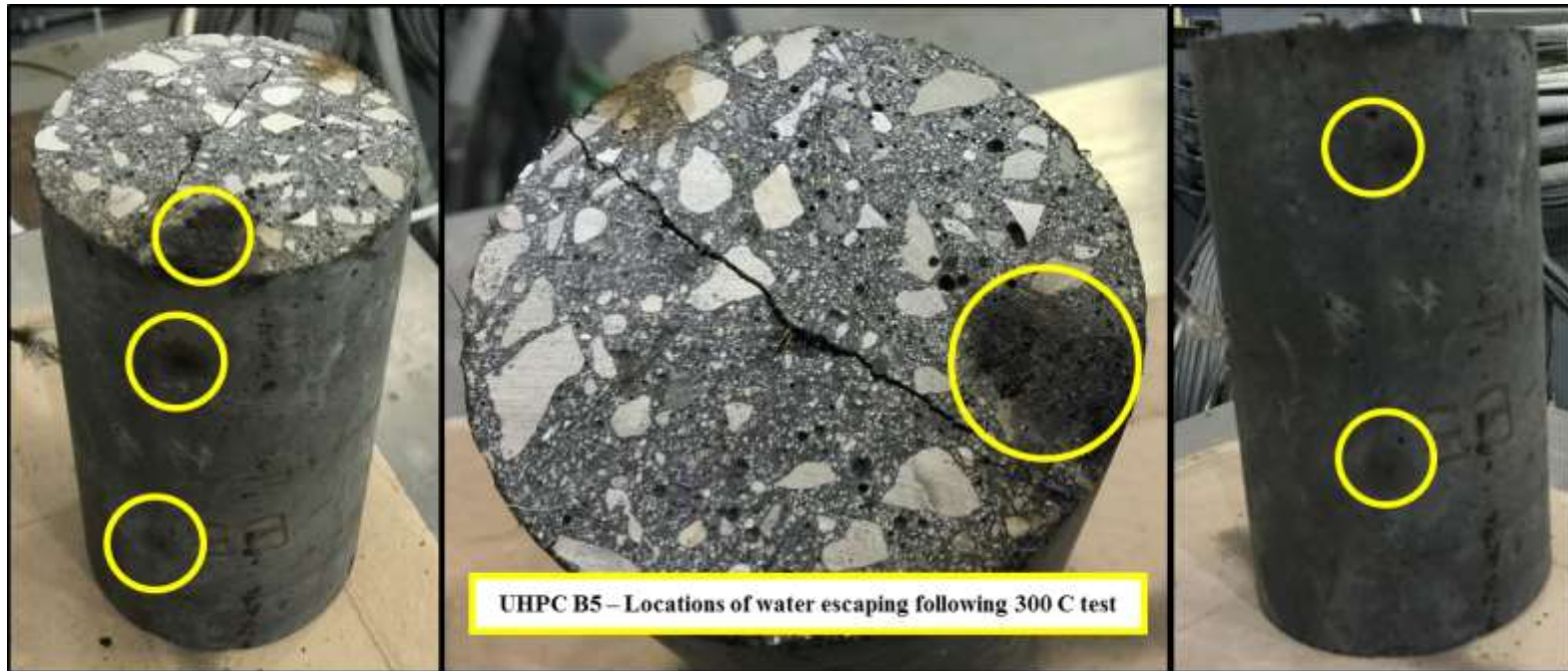
Figure 3.27: Specimen UHPC B5 displaying water escaping concrete following 300°C test
