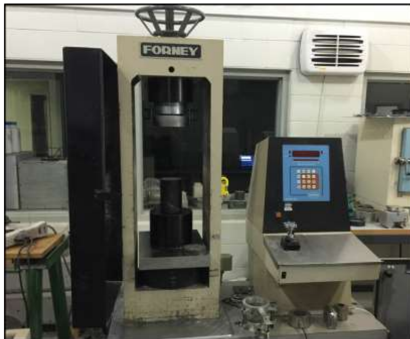
Figure 3.4: Forney load controlled strength testing machine to conduct compressive strength testing as part of this study
