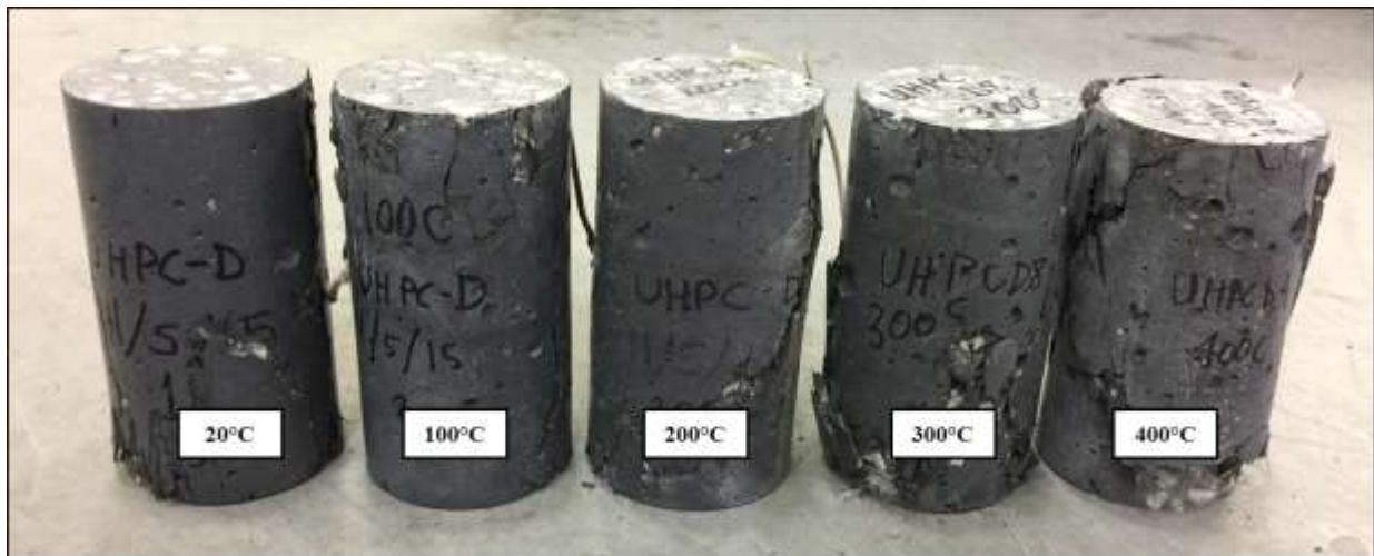
Figure 3.22: Failure modes of UHPC D at respective temperatures
