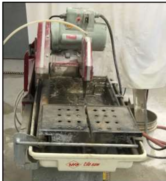
Figure 3.2: Table saw utilized to cut and prepare the concrete cylinders
