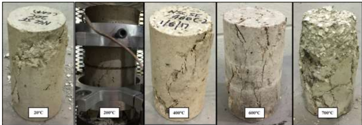
Figure 3.14: Failure modes of NSC-SF at respective temperatures
