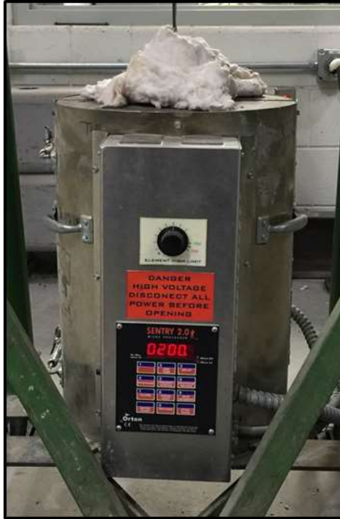
Figure 3.3: Electrical furnace utilized in heating concrete cylinders
