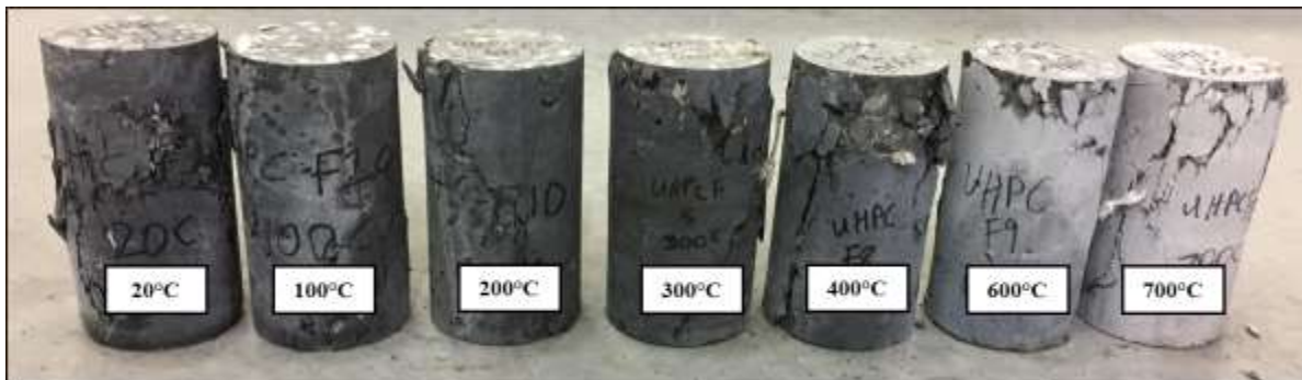
Figure 3.24: Failure modes of UHPC F at respective temperatures
