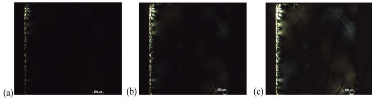
Figure 2. 48 Birefringence images of a 221 \mu\text{m} thick CVD SCD plate with exposure times of (a) 500ms (b) 2000ms and (c) 5000ms [124].
