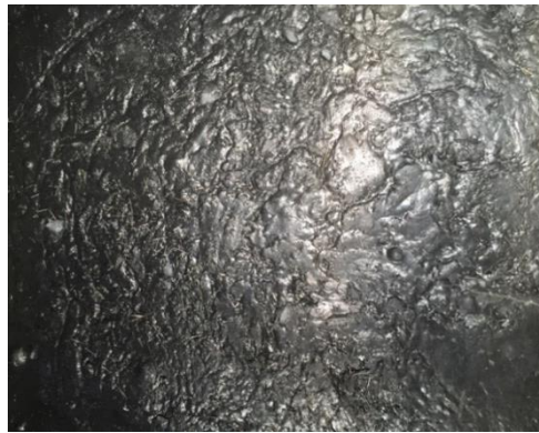
Figure 3.6. Surface appearance of the base UHPC mix, depicting elephant skin formation on the exposed surface.
