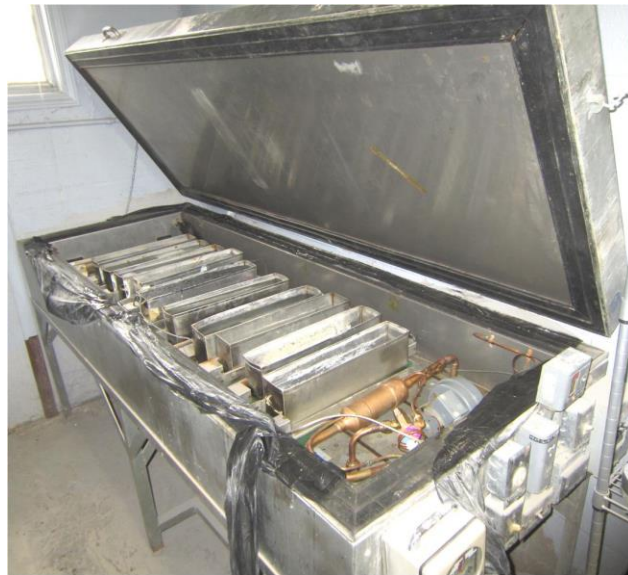
Figure 4.5. Freeze-thaw test chamber.
