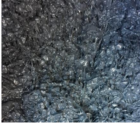
Figure 2.11. The fresh UHPC mix prepared with glued steel fibers.
