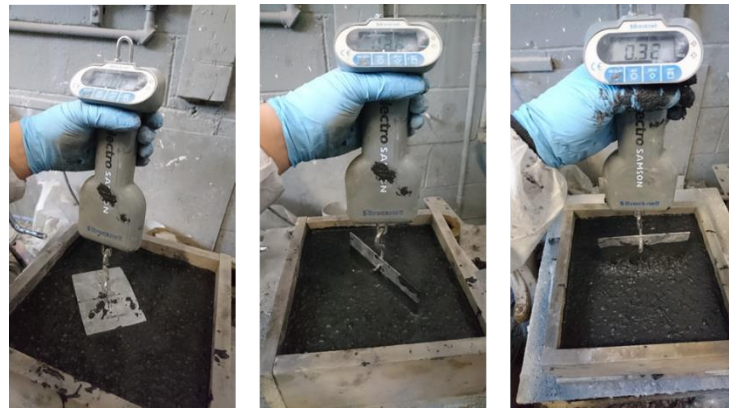
(a) Surface Adhesion Test (b) Push-In Test (c) Pull-Out Test
