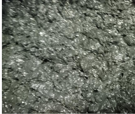
Figure 2.14. The fresh UHPC mix appearance in drum mixer when 25% of fine steel fibers are replaced with medium-sized steel fibers.
