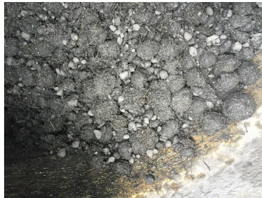
Figure 2.8. The steel fiber balls formed in drum mixer.
