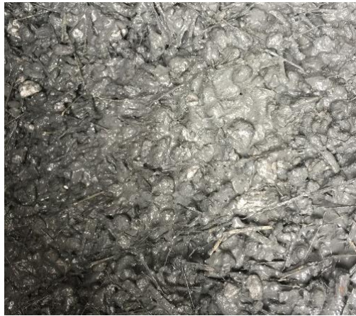
Figure 2.13. The fresh UHPC mix appearance in drum mixer when 50% of fine steel fibers are replaced with medium-sized steel fibers.
