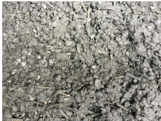
Figure 2.10. The cementitious paste pellets formed in drum mixer for the UHPC mix with carbon fiber reinforcement.
