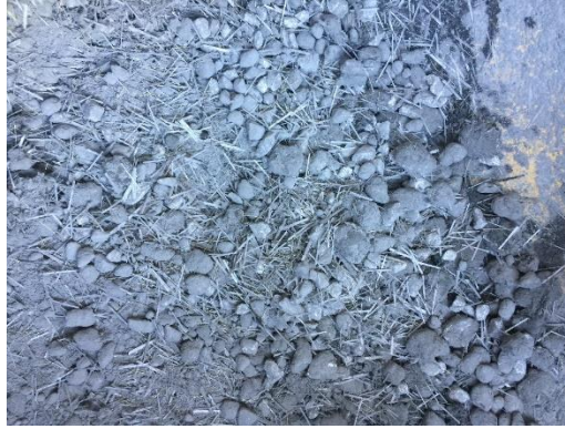
Figure 2.9. The cementitious paste pellets formed in drum mixer for the UHPC mix with glass fiber reinforcement.
