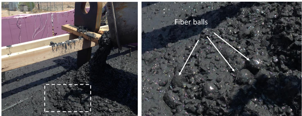
Figure 2.1. Fiber balls produced in large-scale production of UHPC in a ready-mixed concrete truck.
