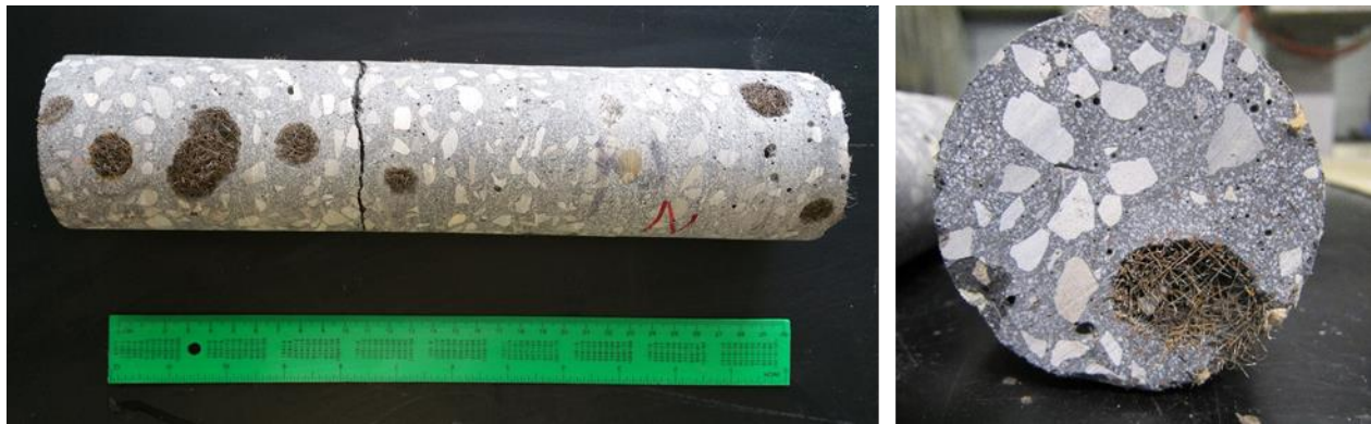
Figure 2.2. Pictures of a UHPC core and its cross-sections taken from a large UHPC placement where mixing was performed in a ready-mixed concrete truck.
