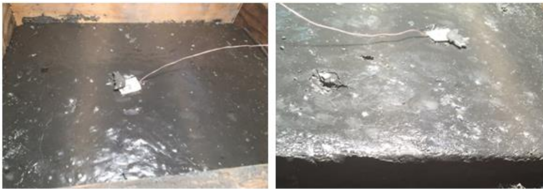
Figure 3.13. Surface appearances of the UHPC mix incorporating polypropylene fibers prior to and after exposure to air flow and radiation.
