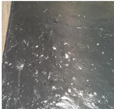
Figure 3.18. Surface appearance of the UHPC mix incorporating cellulose ether after exposure to air flow and radiation.
