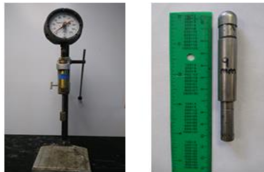
Figure 3.5. The penetration test apparatus and test probe.
