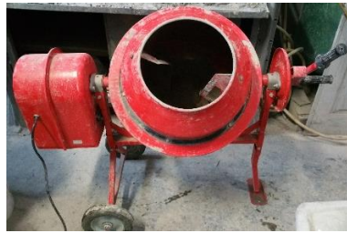
Figure 2.4. The laboratory-scale rotary drum mixer used in this investigation.
