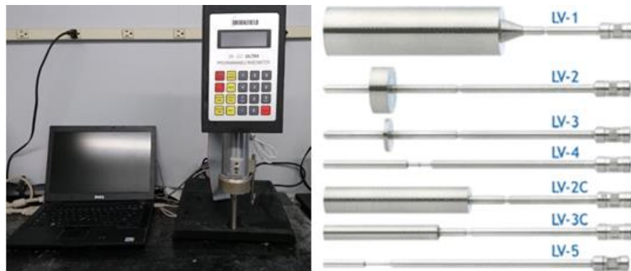
Figure 2.7. The rheometer and the spindles (LV-5 was selected after preliminary trials) used in this investigation.
