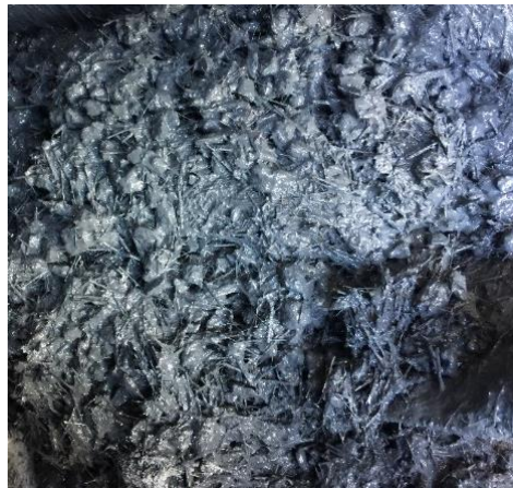
Figure 2.12. The fresh UHPC mix appearance in drum mixer when 50% of fine steel fibers are replaced with coarse (hooked) steel fibers.
