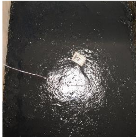
Figure 3.8. Surface appearance of the UHPC mix incorporating carbon fibers during the test.
