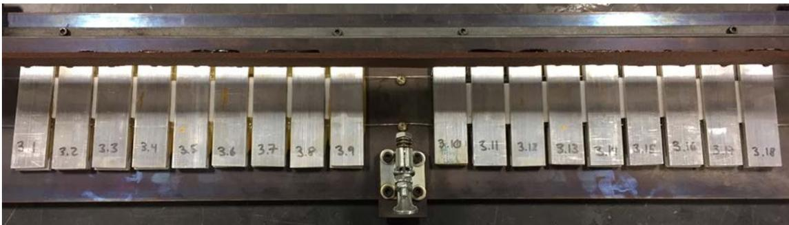
Figure 3-11. Fixture for the manufacture of “sandwich” lap joints after thermal cycling
