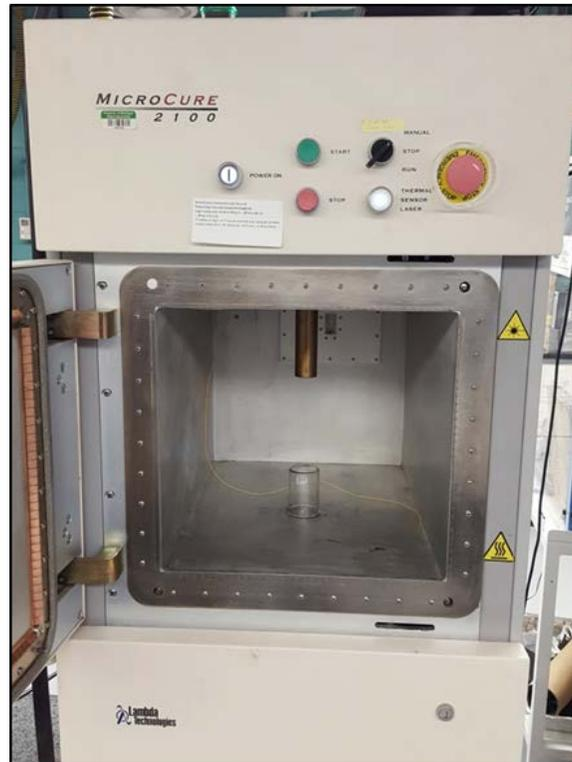
Figure 5-1. MicroCure 2100 variable frequency oven showing chamber, IR temperature probe, and glass sample stand
