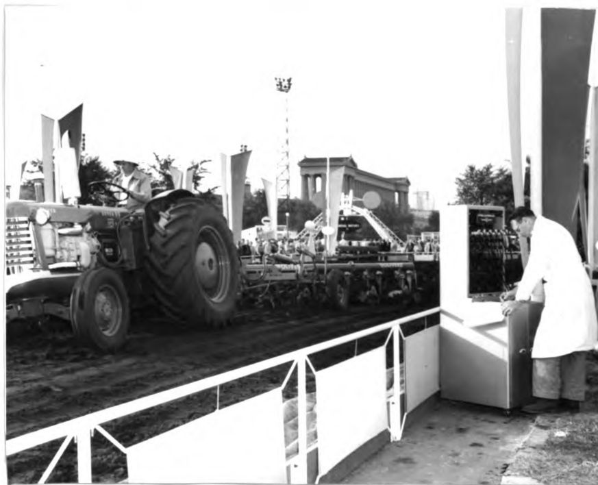
Fig. 8. Recording Soil Pressures Under Tractor and Plow
