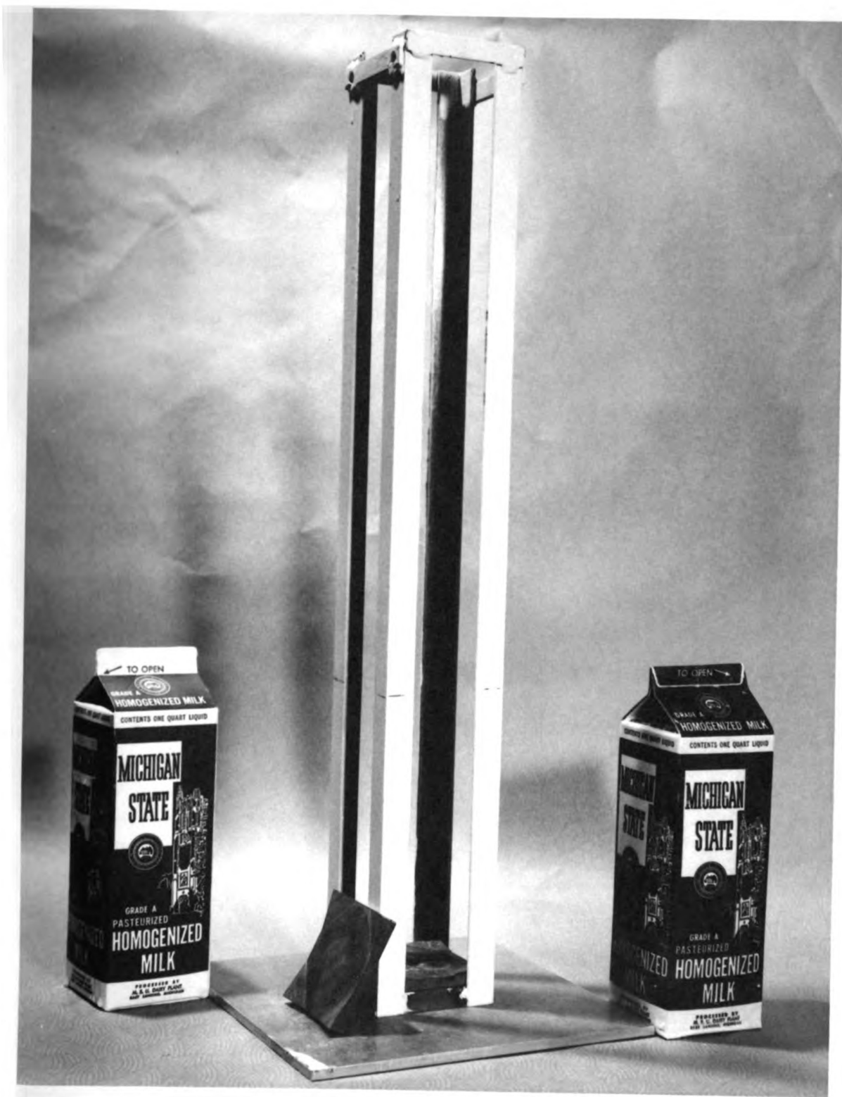
FIGURE 5. Standard drop test apparatus, experimental milk carton (l.) and milk carton in present use (r.)
