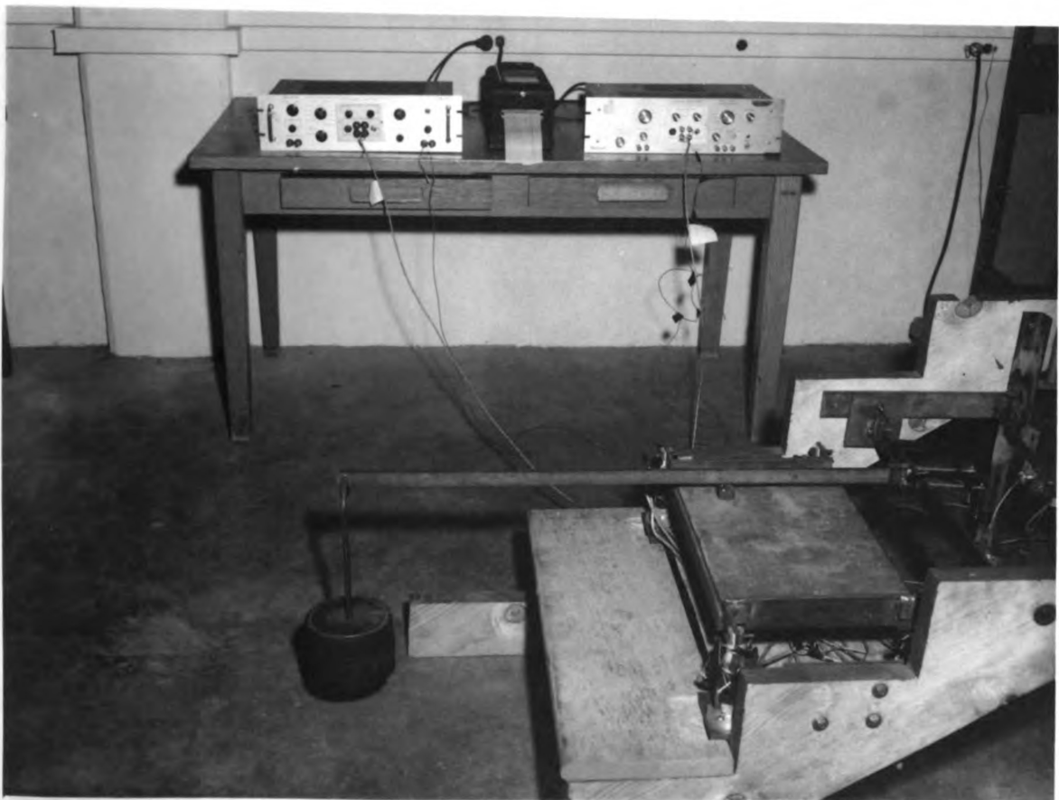
Figure 7: Calibrating the force plate for vertical forces and the coordinate system.
