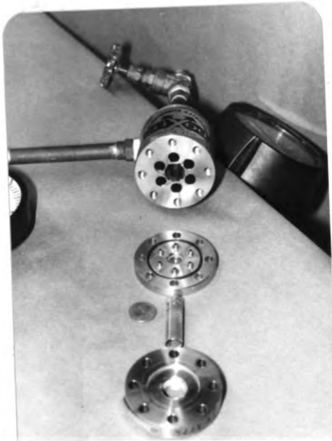
Figure 3.5. Photographs of the Dorrclone connections and cluster design.
