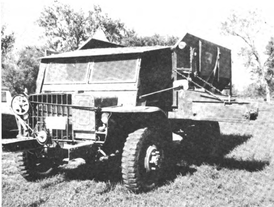
Fig. 22. Power feeder truck made from used parts.
