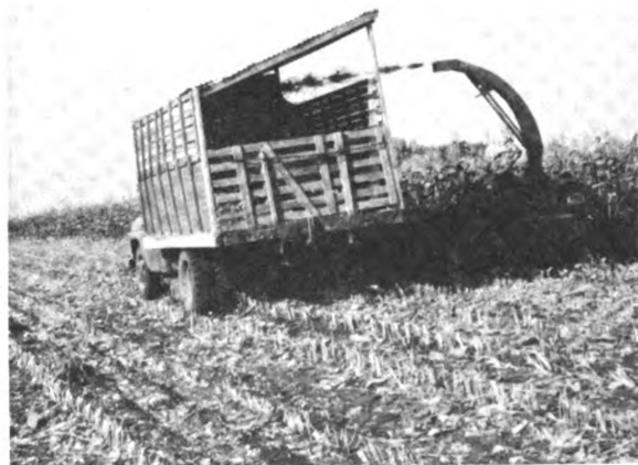
Fig. 15. Truck with roof to prevent wind loss while traveling being loaded with corn silage.
