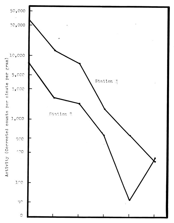
Figure 9. Activity of periphyton at Stations 12 and 14. The substrates remained in the water during isotope treatment. Counts were corrected for background and decay.
