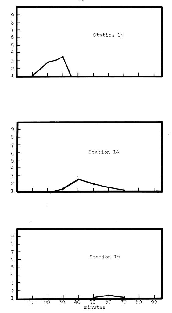
Figure 5. Continuous total water activity at collecting Stations  $^{\rm P}$ , 11 and 12 for July 6 and July 7, 1960. Counts were corrected for background and decay.
