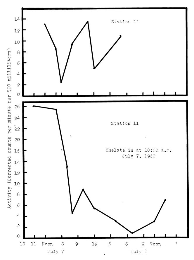
Hand-collected samples were taken immediately after the addition of the chelate. The samples were taken on July 7, 1960 at Station 12 at five-minute intervals starting at 10:50 a.m. for the first hour and then at ten-minute intervals. The same procedure was followed at Station 14 with the starting time at this station of 11:07 a.m. of the same day.
