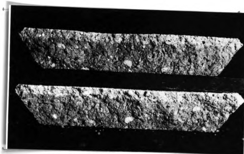
NO COMPOUND - CURED IN CABINET WATER LOSS - 31.3 GRAMS
