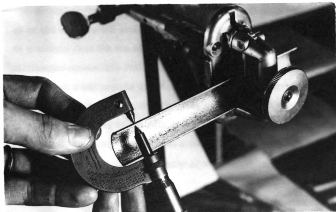
Figure 6. The Pointed Micrometer in Use
