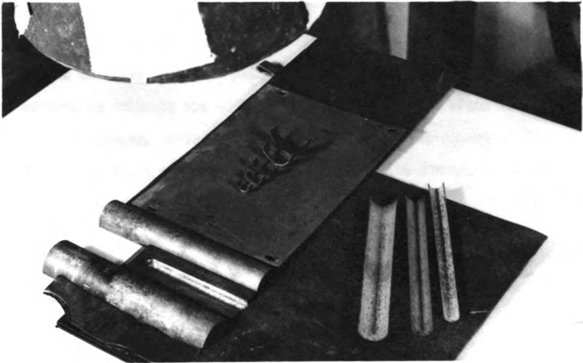
Figure 7. Set-up for Making Radiographs
