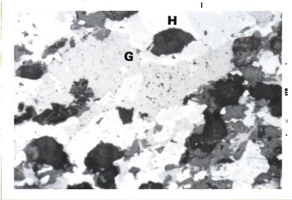
Figure 16.--Hydration of hematite (H) to goethite (gray) in brown ore. (Polished Section; 350X)
