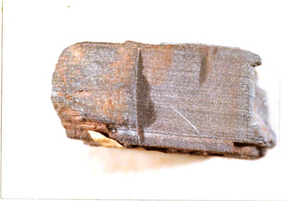
Figure 13.--Siliceous blue biscuit, mainly hematite and silica. 1X
