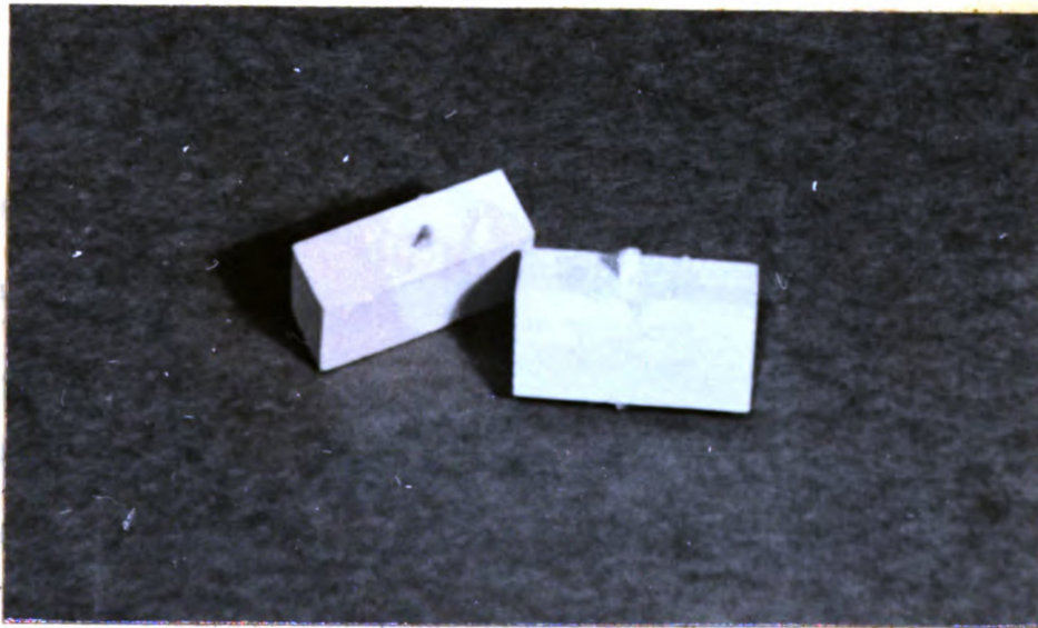
Fig. 11-B. Typical failure of withdrawal specimen above linear portion of curve.
