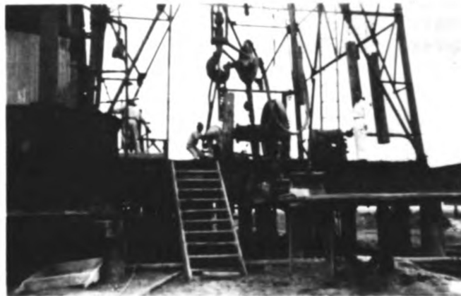
Plate 3.- A standard rotary drilling machine used in deep wells in the Tigre field (Santa Elena), Ecuador.
