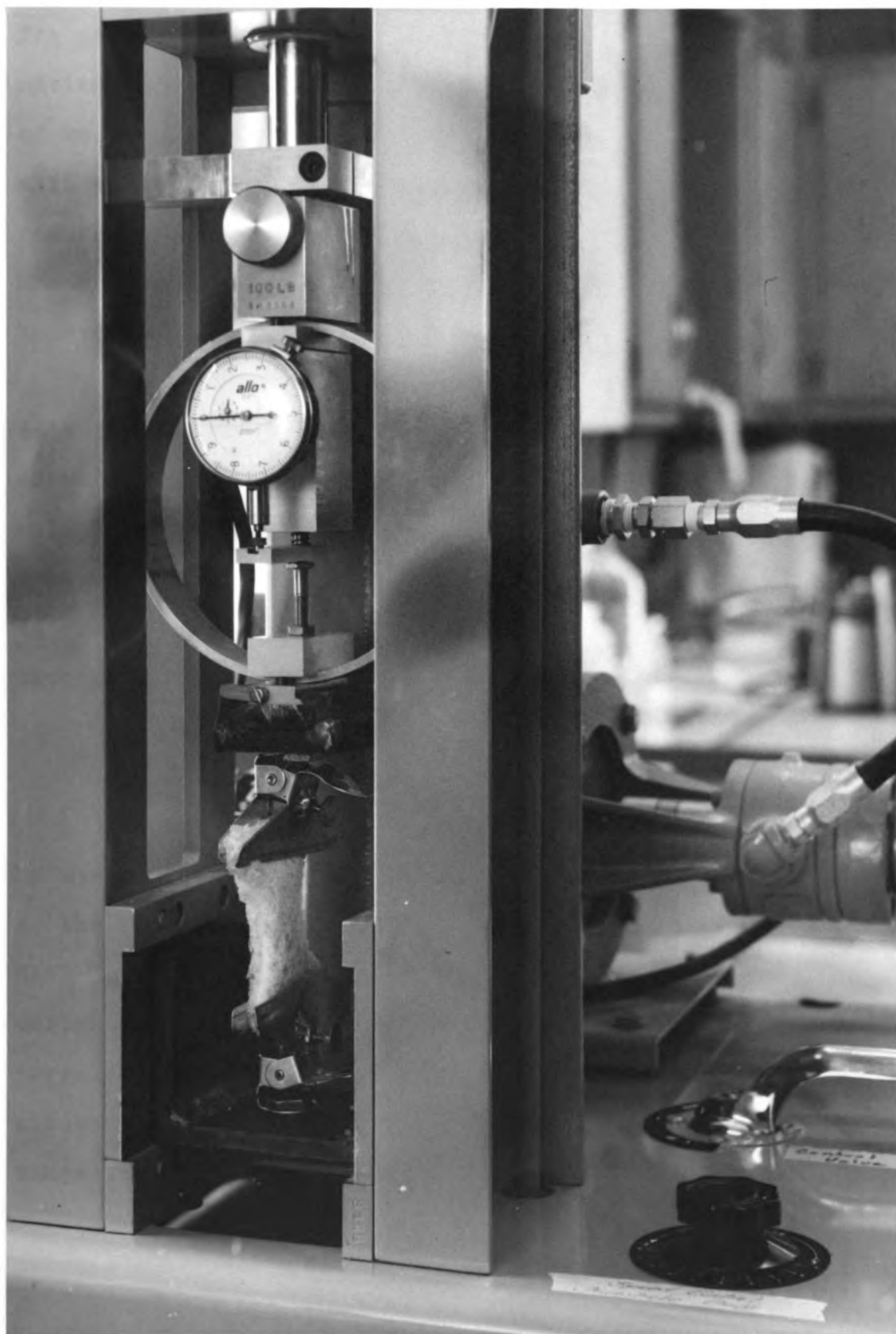
Figure 5. Measurement of the Tensile Strength of Angel Cake by the Shear Press.
