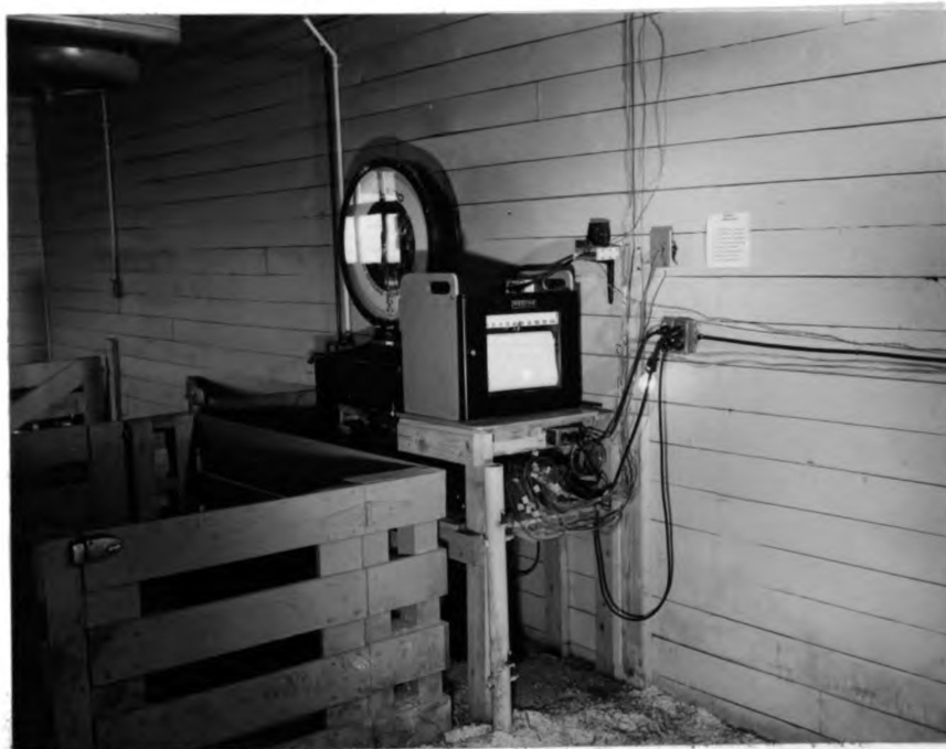
Fig. 5. Instrument location from door leading to solar wing. Shows respective location of potentiometer, switching box, time clock, transformer, and eight point plug. Sign on wall explains location of different thermocouples being recorded.
