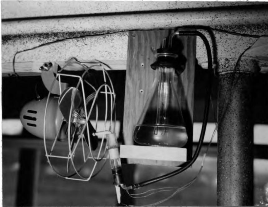
Fig. 16. Relative humidity measuring unit. Water level in large glass tube was always at same height because small tube in Erlenmeyer flask opens to atmosphere. Fan is eight inch household fan.
