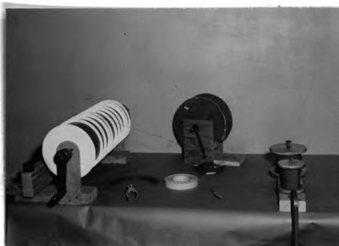
Fig. 12. Drum with crank was used to wind up wires which made thermocouple strings. Drum revolution counter to meter out correct length of wire was located at front edge behind drum.
