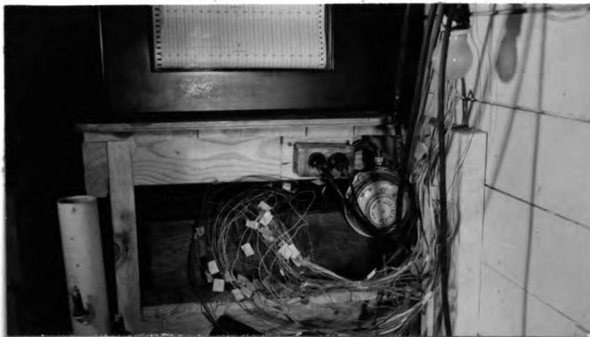
Fig. 7. Location of switching box and time clock below potentiometer. Light-bulb to which thermocouple lead was attached appears in upper righthand corner.
