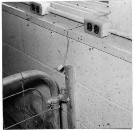
Fig. 15. Typical location of thermocouple junction along outside walls.
