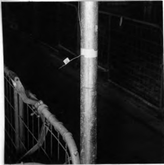
Fig. 14. Typical location of thermocouple junction on every other post along alley of both wings.
