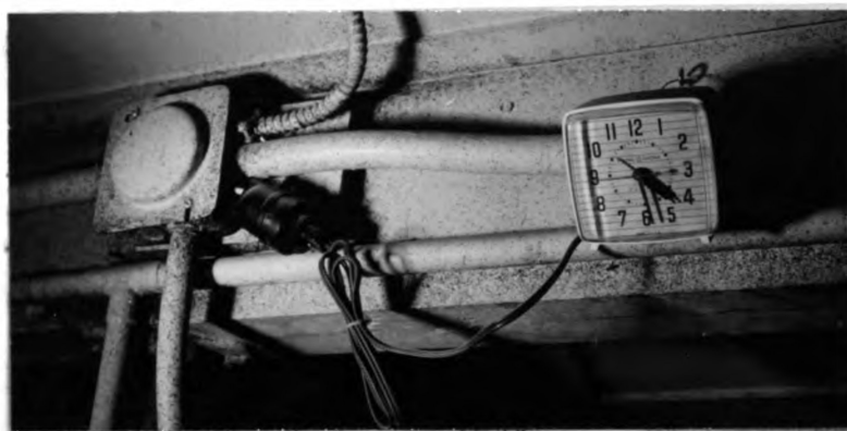
Fig. 19. Clock, connected in parallel with heater fan, was used to record total hours of heater fan operation.
