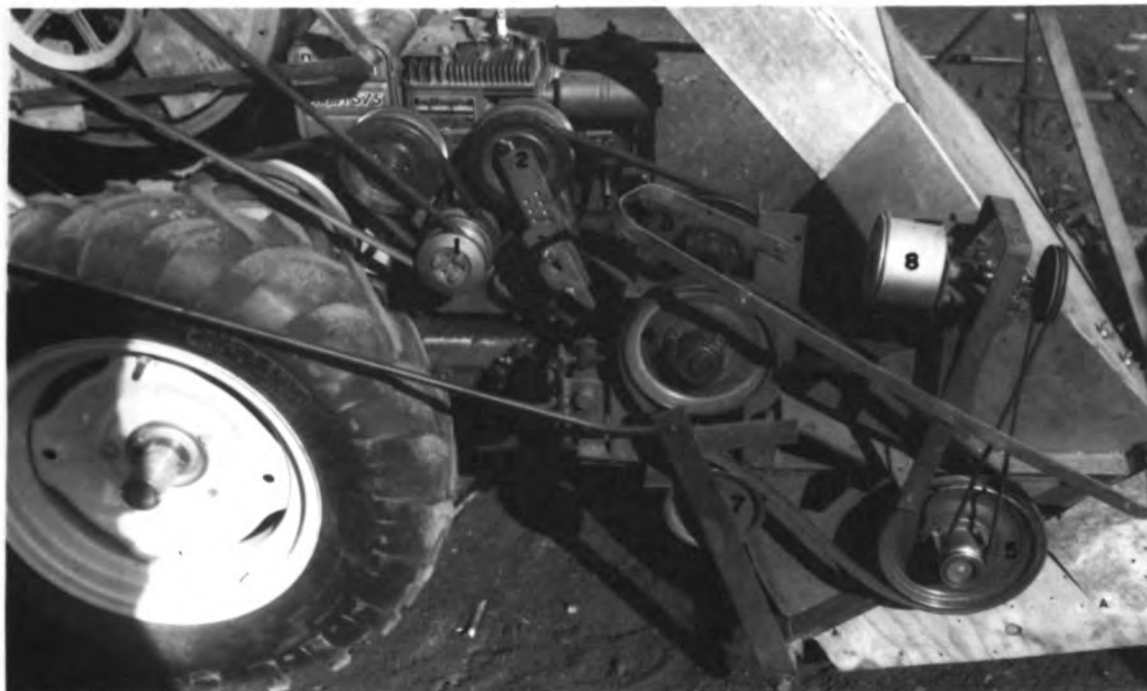
Fig. 3. Right side of the combine with transmission shield removed: transmission pulleys to the flail shaft are 1, 2, 3, 4, 5; 6 is the crank for the speed changer pulley 2; 7 is idle pulley clutch, and 8 is the tachometer.
