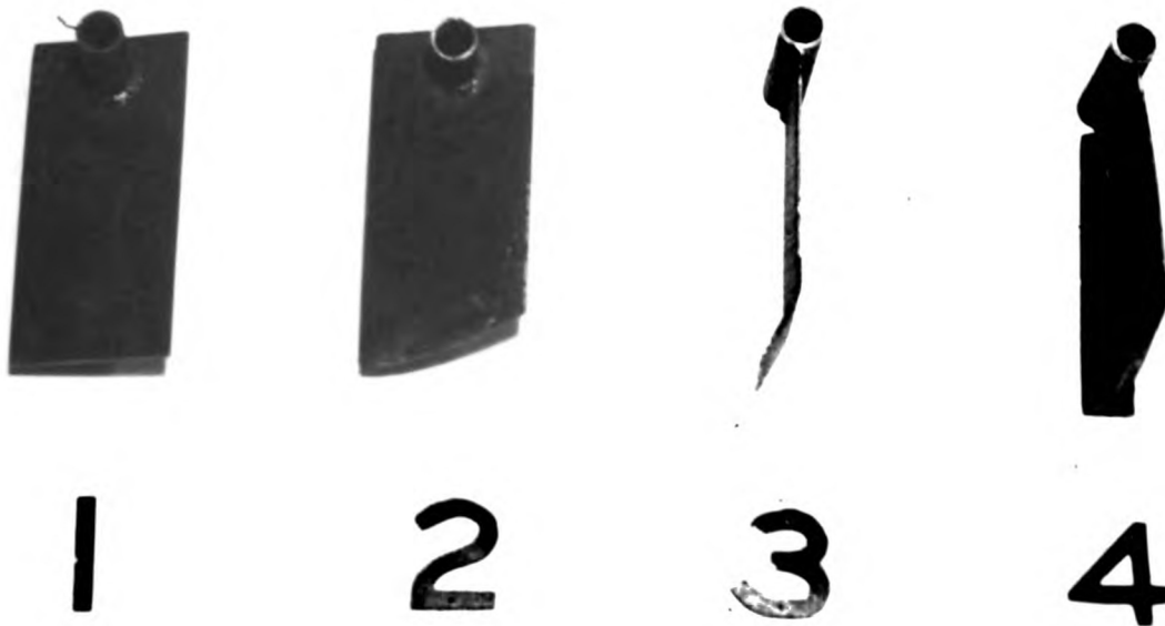
Fig. 6. Side view of the flails: (1) propeller flail, (2) modified propeller flail, (3) direct throwing flail, and (4) modified direct throwing flail.
