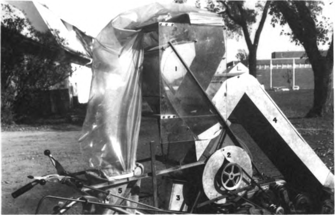
Fig. 7. (1) The swirl-chamber, (2) fan with fan shutters, (3) grain box, (4) duct from the cutterheads, (5) burlap sack.
