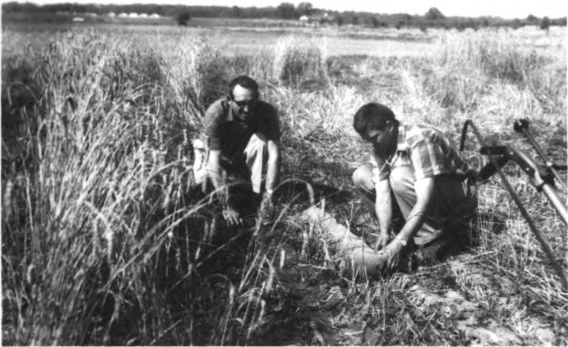
Fig. 15. Dr. W. F. Buchele and author rolling the two sheets of canvas which were placed on each side of the row to catch the cutterhead losses of grain.
