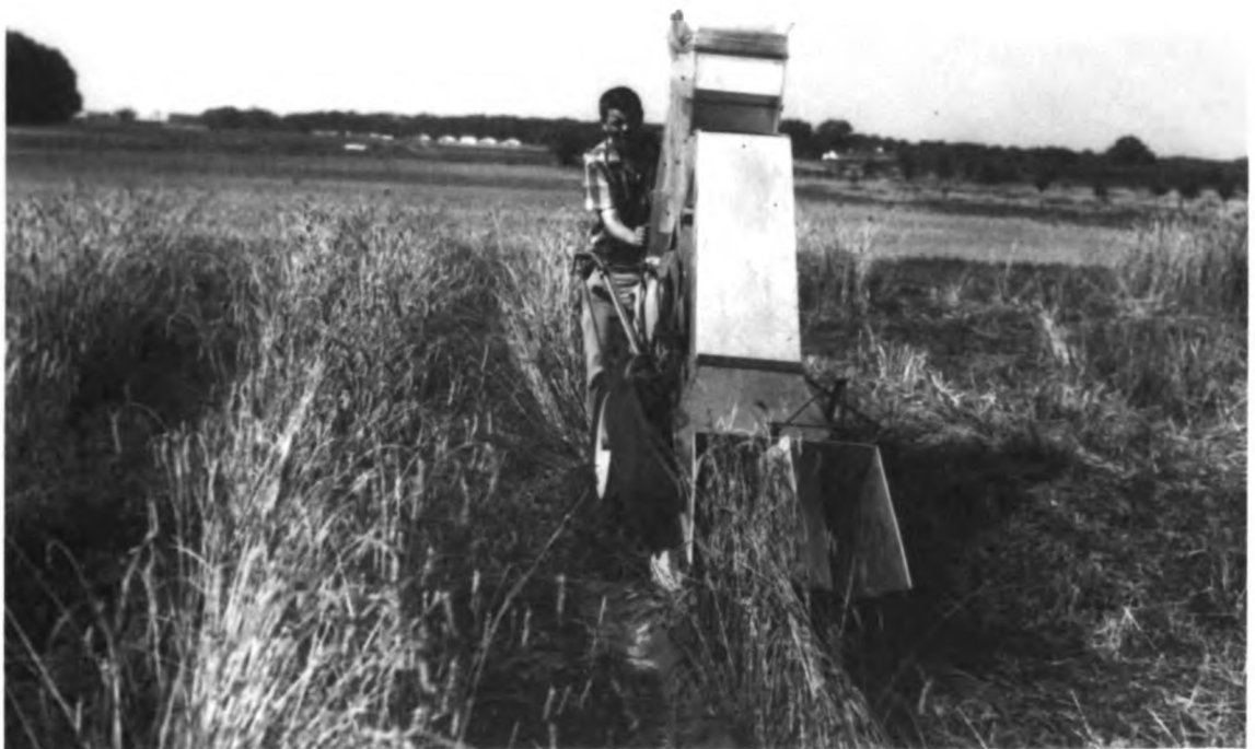
Fig. 14. Right cutterhead harvesting a single row of wheat lodged so that the heads entered the cutterhead first.
