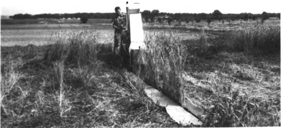
Fig. 13. Right cutterhead harvesting a single row of standing wheat.
