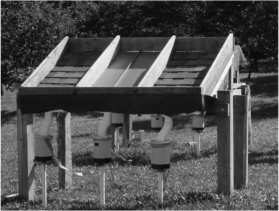
Conventional roofing partitions draining into separate tipping bucket measuring devices (Photo courtesy of Cronk 2010).
