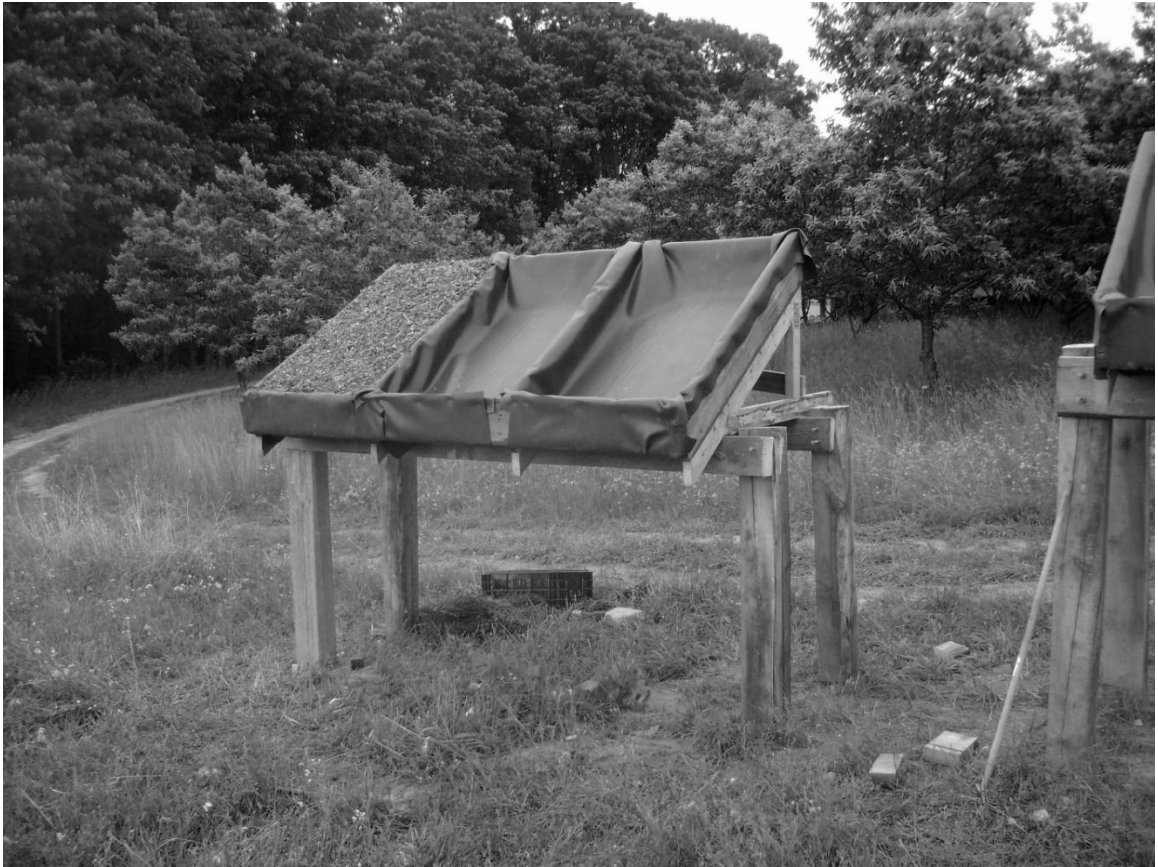
Photo of .045mm EPDM rubber membrane used for waterproofing in study plots (Photo courtesy of Cronk 2010).
