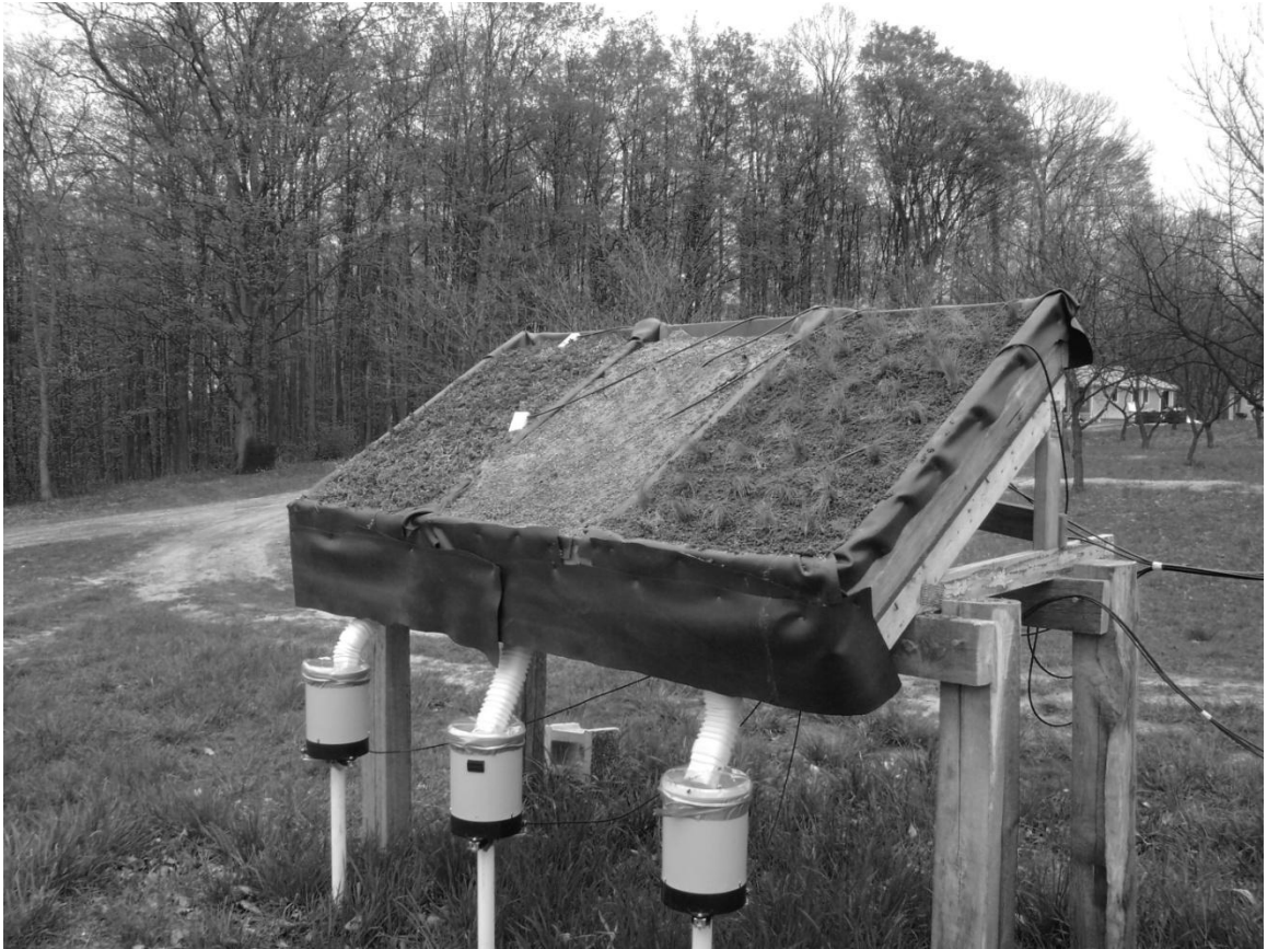
Green roof partitions draining to separate tipping bucket measuring devices (Photo courtesy of Cronk 2010).
