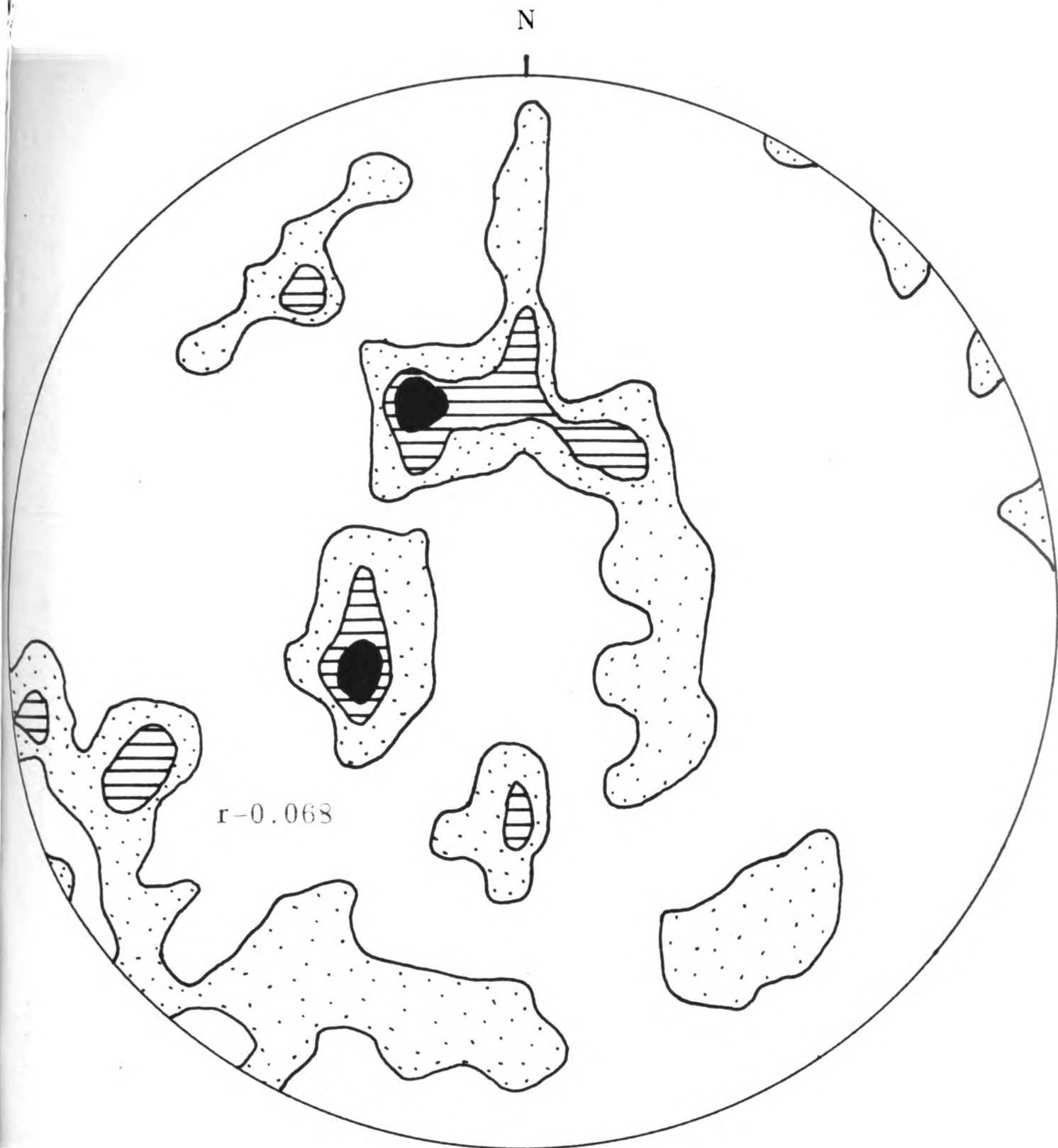
Figure 24. 330 dolomite axes from sample H contours 3-2.1-1.2 percent, plotted on the lower hemisphere of a Schmidt equal-area net.
