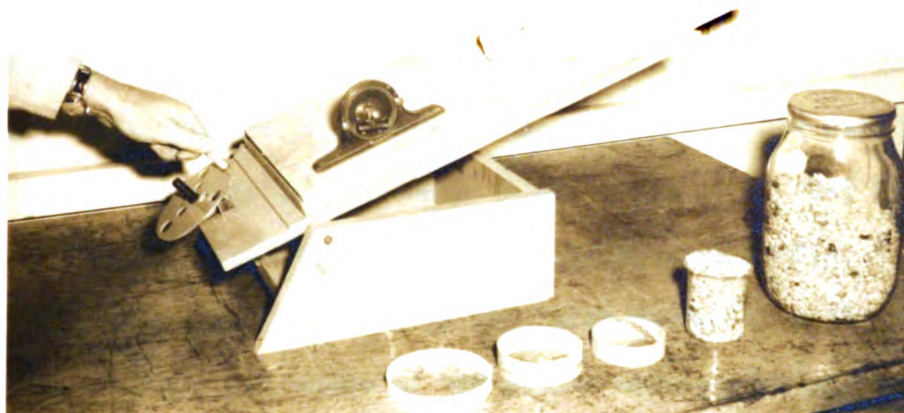
Fig. 2. Tilting Table Used for Coefficient of Friction Determinations.
