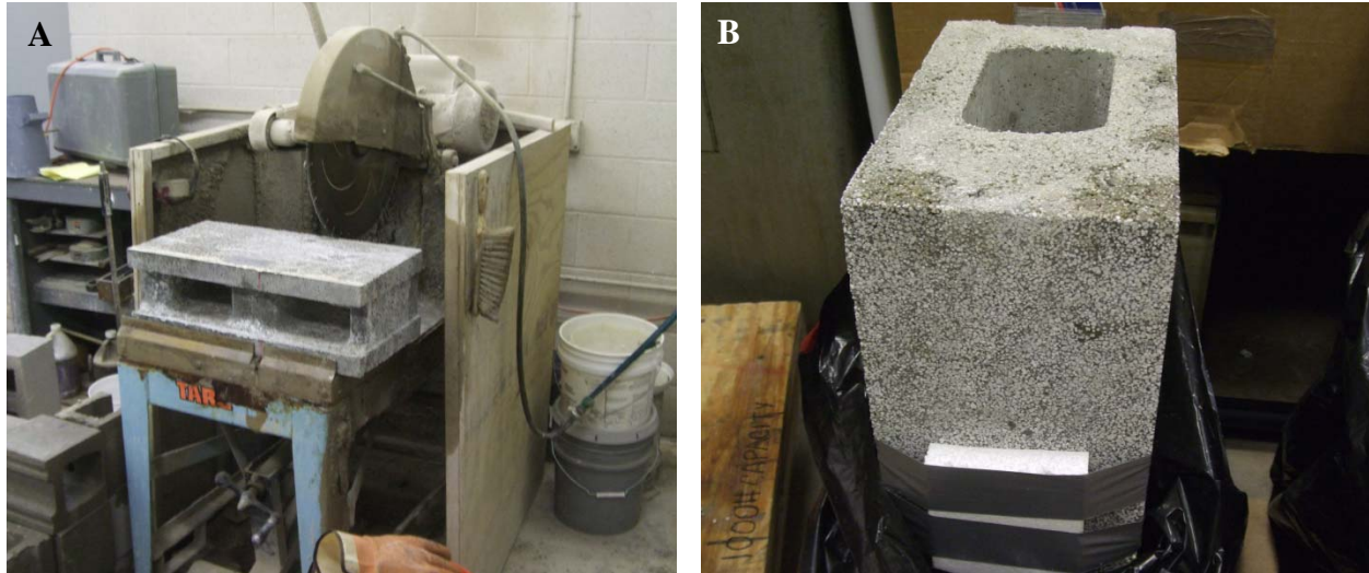
Figure 4.11: Prism test preparation. (a) block ready for cutting on masonry saw; (b) recently stacked prism prior to grouting.
