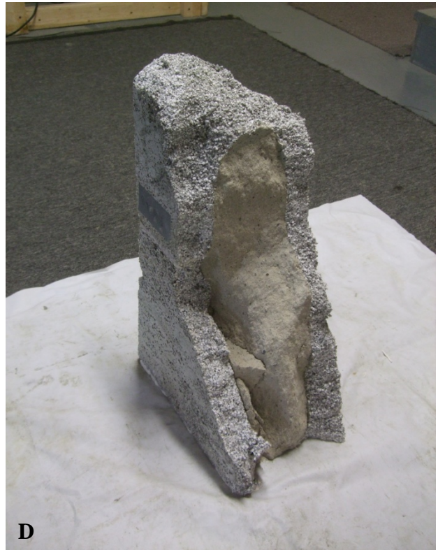
Figure 4.12: Prism testing. (a) recently capped prisms; (b) hydraulic testing equipment; (c) prism after testing with signs of failure in the face; (d) remaining segment of prism with block material still intact with part of the core.
