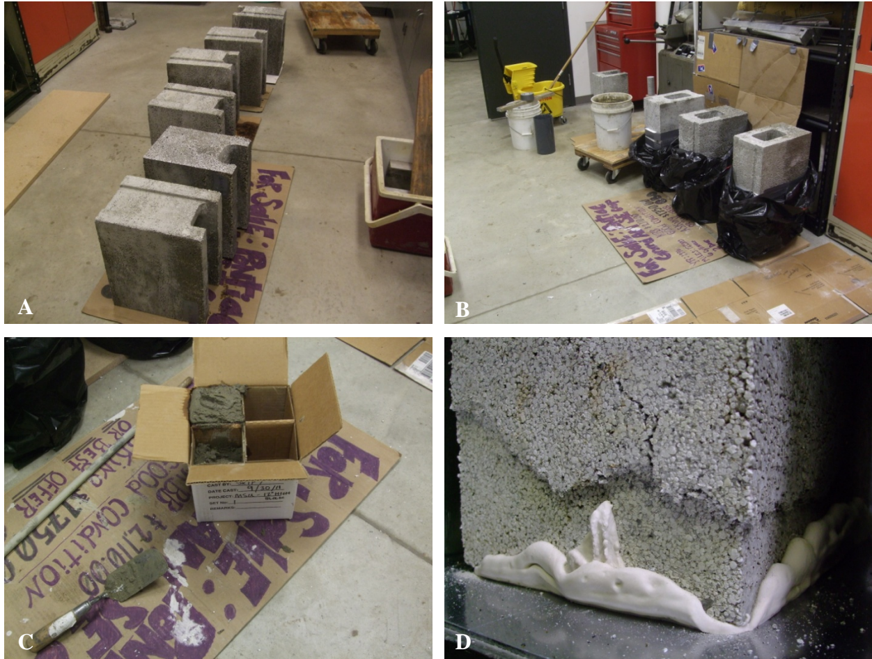
Figure D.11: Additional images of masonry prism preparation and testing. (a) blocks after being cut in half for prism assembly; (b) assembled prisms ready to received grout; (c) grout prism sample to ensure grout has reached specified strength; (d) close-up of visible movement of part of the prism after failure.
