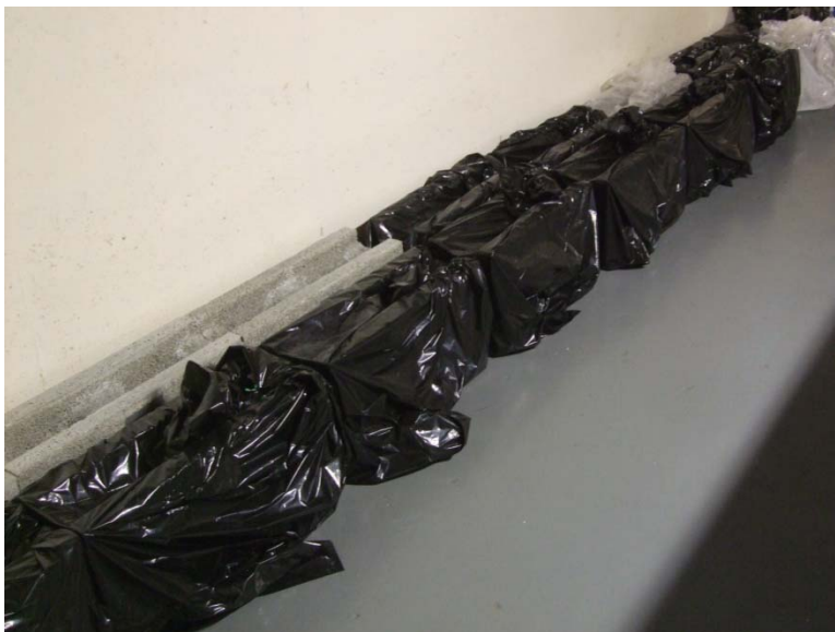
Figure 4.10: Curing method for the blocks.
