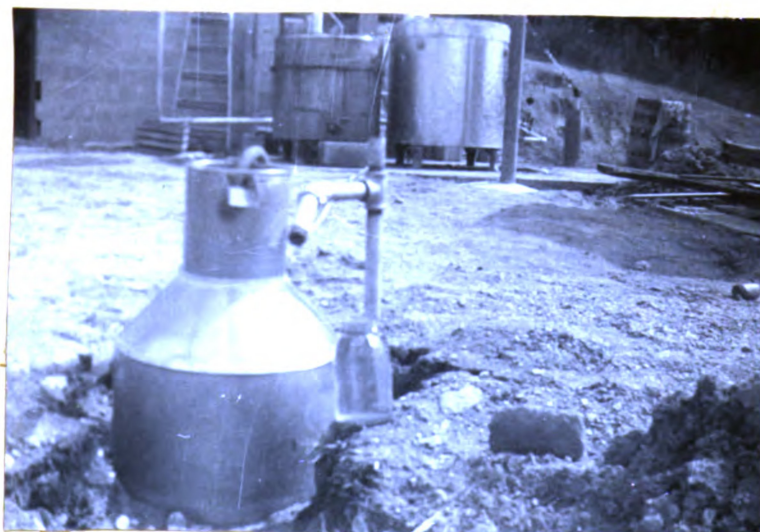
Figure 15. The receiver. Here it is placed in series with the first receiver to test whether any oil is passing through the drain of the first receiver. Only non-measurable traces were found under proper operating conditions. The quart bottle is used to measure the steam flow by weighing the amount of condensate caught in a period of time. Example: two pounds caught in 30 seconds would give a steam flow of 240 pounds per hour.
