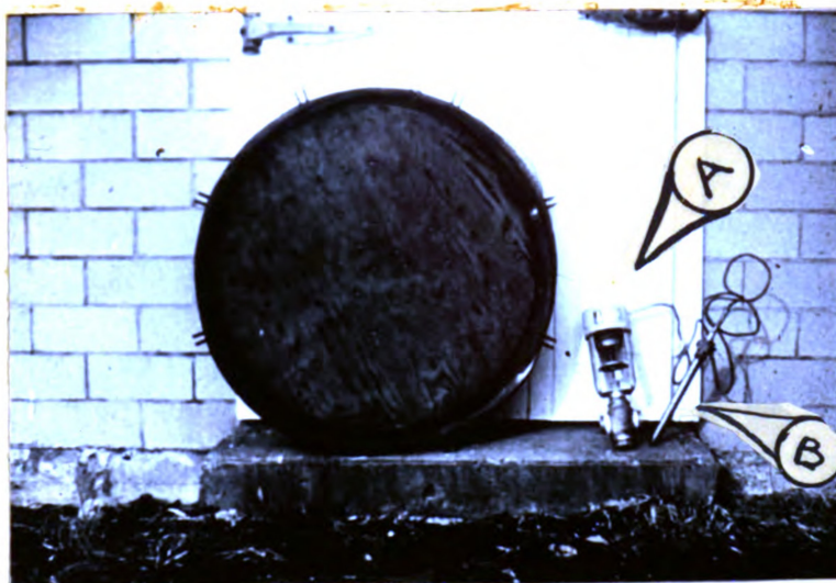
Figure 9. Photograph of marine plywood cover taken in January 1955. The lid has been exposed to the weather and has been used with steam on 176 mint distillation trials. As yet their is no sign of deterioration except a discoloration of the wood. To the right is the condensate temperature control valve (A) and its sensing elements (B).
