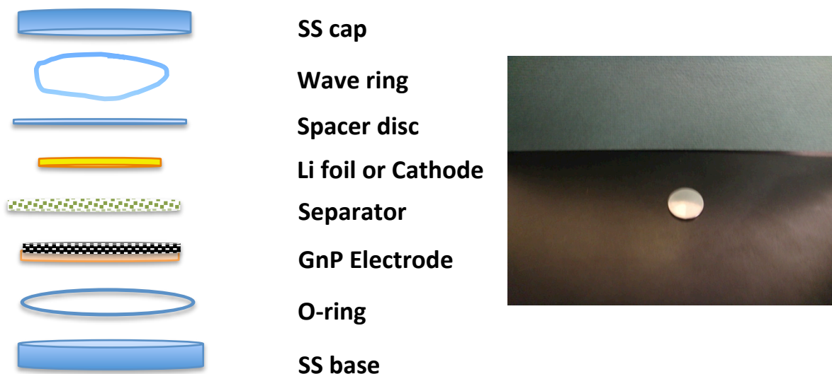
Figure 3-3: Schematic and pictures of Two-electrode Coin cell
