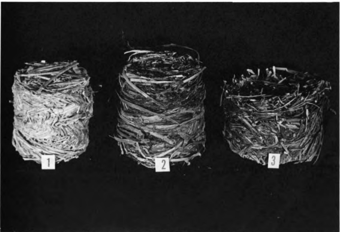
FIGURE 24. ILLUSTRATION OF THE BASIC STRUCTURAL DIFFERENCES BETWEEN WAFER MADE WITH: 1. PLUNGER DEVICE, 2. ROLLING APPARATUS, 3. PLUNGER DEVICE WITH PREORIENTED HAY
