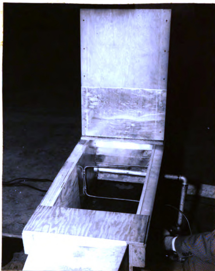
Fig. 15. Steam Entering the Air Duct
