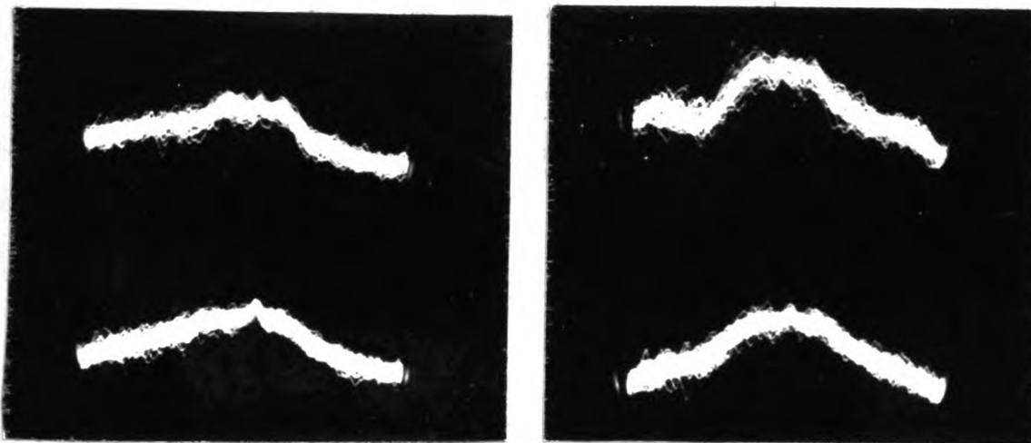
Figure 11. Photographs of the proton resonance signal from single crystals of hypo.
