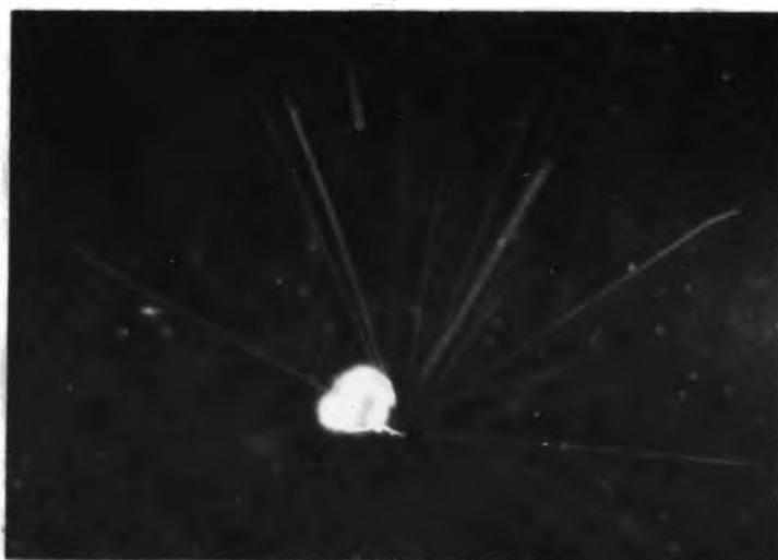
Fig. 18. \alpha tracks at an expansion ratio of 1.125 P = 9\frac{1}{2} cm of Hg
