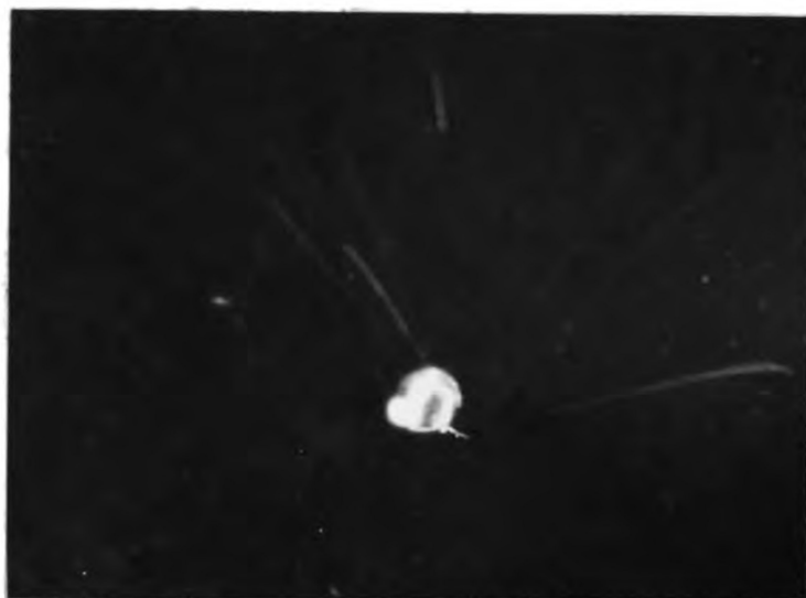
Fig. 17. \alpha tracks at an expansion ratio of 1.118 P = 9 cm of Hg
