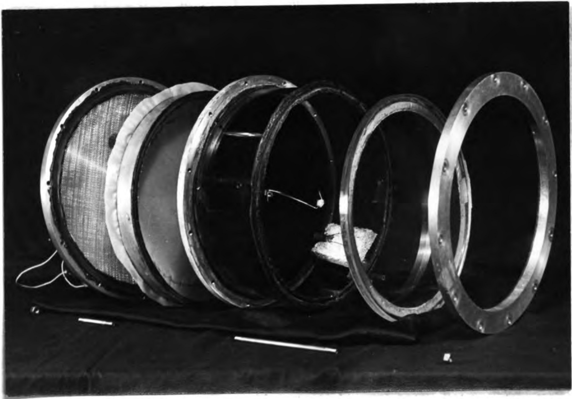
Fig. 4. Exploded view of the cloud chamber.
