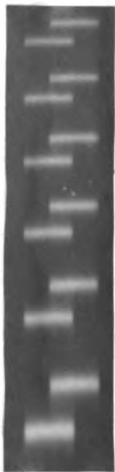
16 min. exposure \text{Hg}^{198} 5770, 5790A NBS Meggers \text{Hg}^{198} Electrodeless
