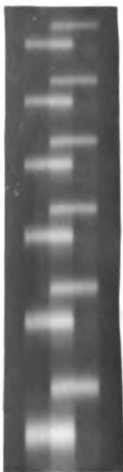
8 min. exposure \text{Hg} 5770, 5790A (natural) Electrodeless Lamp No. 27
