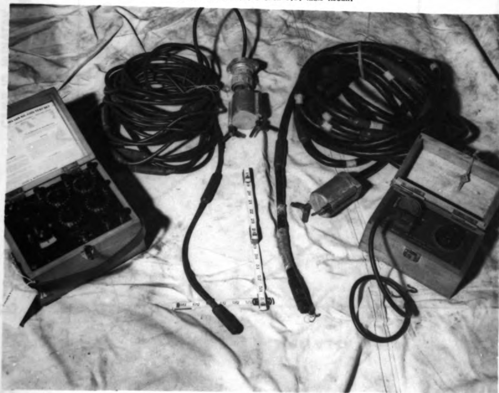
FIG.6 WHEATSTONE BRIDGE, SELECTOR SWITCH AND THERMISTOR GLACIO-THERMAL CABLES USED ON THE JUNEAU ICEFIELD RESEARCH PROGRAM, 1960 AND 1961.
