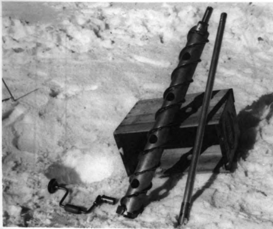
FIG.5 S.I.P.R.E. 5 INCH O.D. HAND AUGER.
