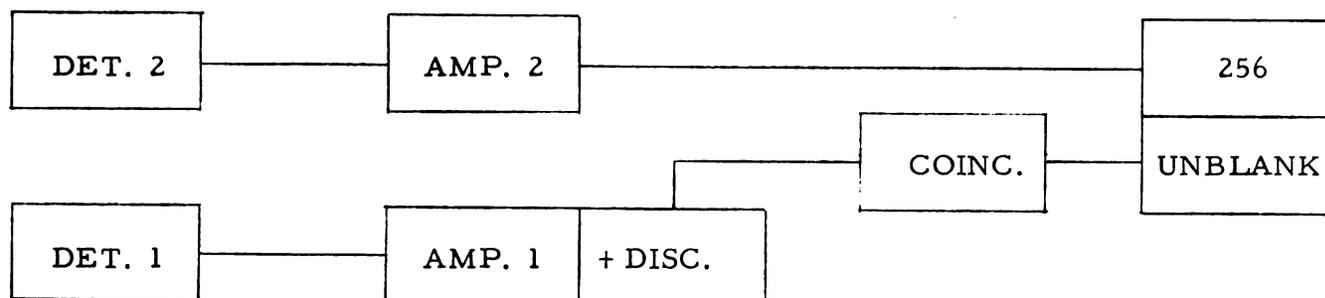
Figure III. Block diagram of circuit used to obtain coincidence correction. "Det." signifies detector, "Amp." amplifier, "+Disc." the positive discriminator output of the amplifier, "Coinc." the coincidence circuit, "256" the 256-channel pulse height analyzer.
