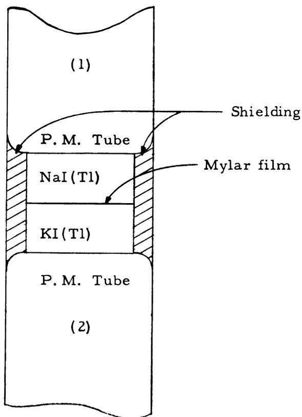
Figure II. Cross-section of the source and light-collection portion of detectors 1 and 2.
