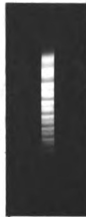
Figure 10 Fabry-Perot Interference Fringes
