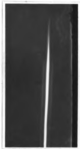
Fig.6. Diffraction picture of traveling sound waves. A sound absorber has removed the standing wave structure.
