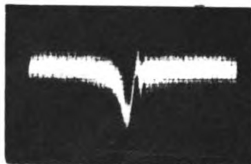
SODIUM STEARATE TRANSITION POINT FROM LIQ. TO LIQ. CRYSTAL STATE
