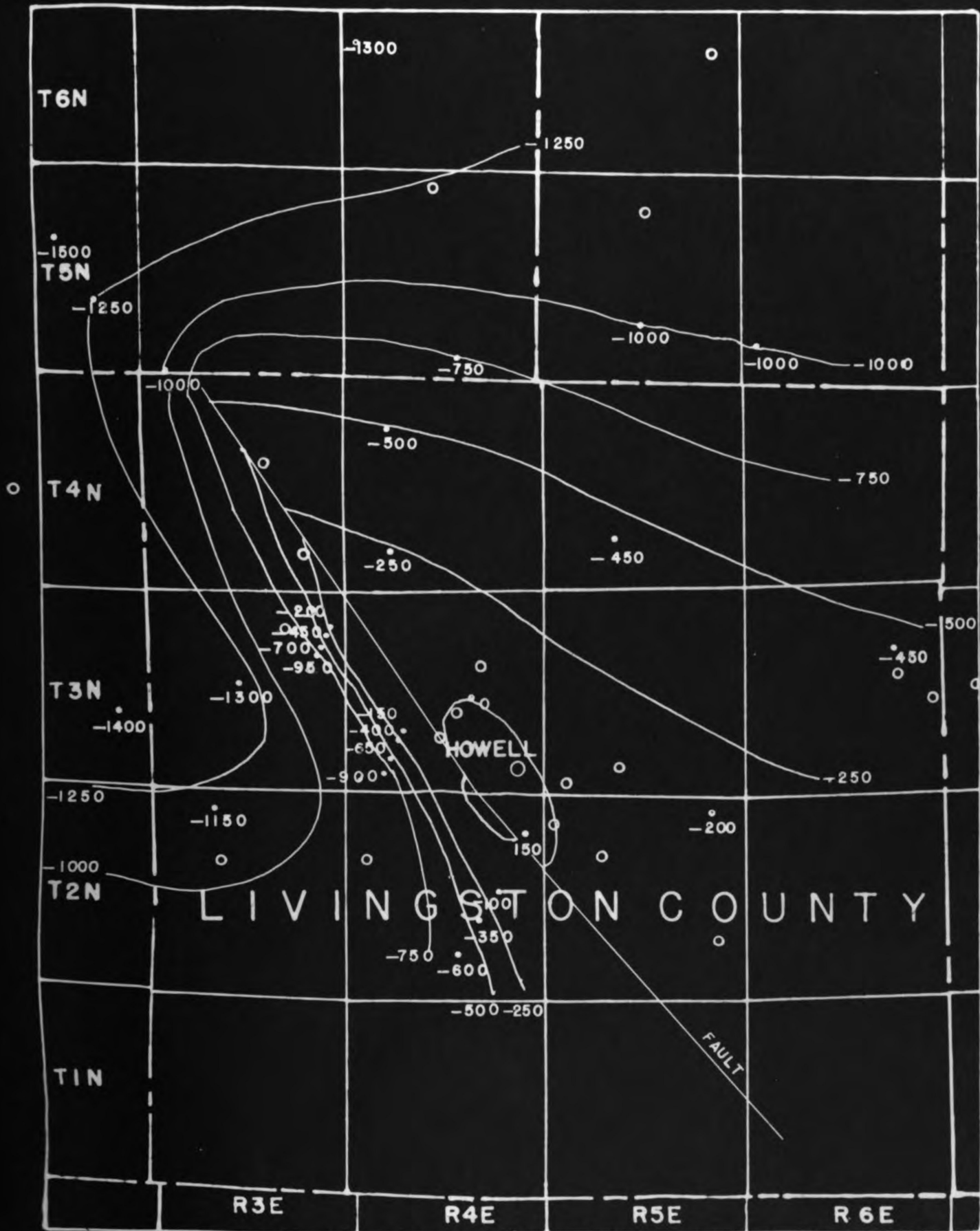
FIGURE 7. STRUCTURE MAP ON TOP OF THE DUNDEE LIMESTONE DETERMINED BY SUBTRACTING THE SUNBURY-DUNDEE ISOPACHOUS INTERVAL (FIGURE 9A) FROM THE BEREA STRUCTURE (FIGURE 4) CONTOUR INTERVAL 250 FEET 0 SCALE 4 MILES
