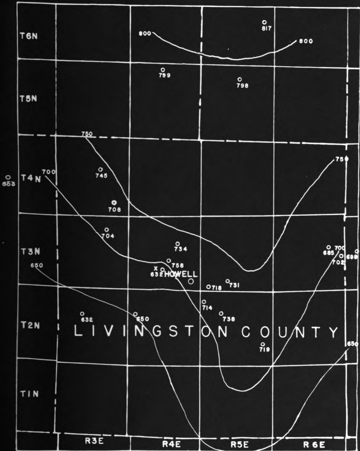
FIGURE 9B. ISOPACHOUS MAP SHOWING THE INTERVAL BETWEEN THE BASE OF THE SUNBURY SHALE AND THE TOP OF THE DUNDEE LIMESTONE CONTOURED WITHOUT A FAULT ISOPACHOUS INTERVAL 50 FEET SCALE 4 MILES
