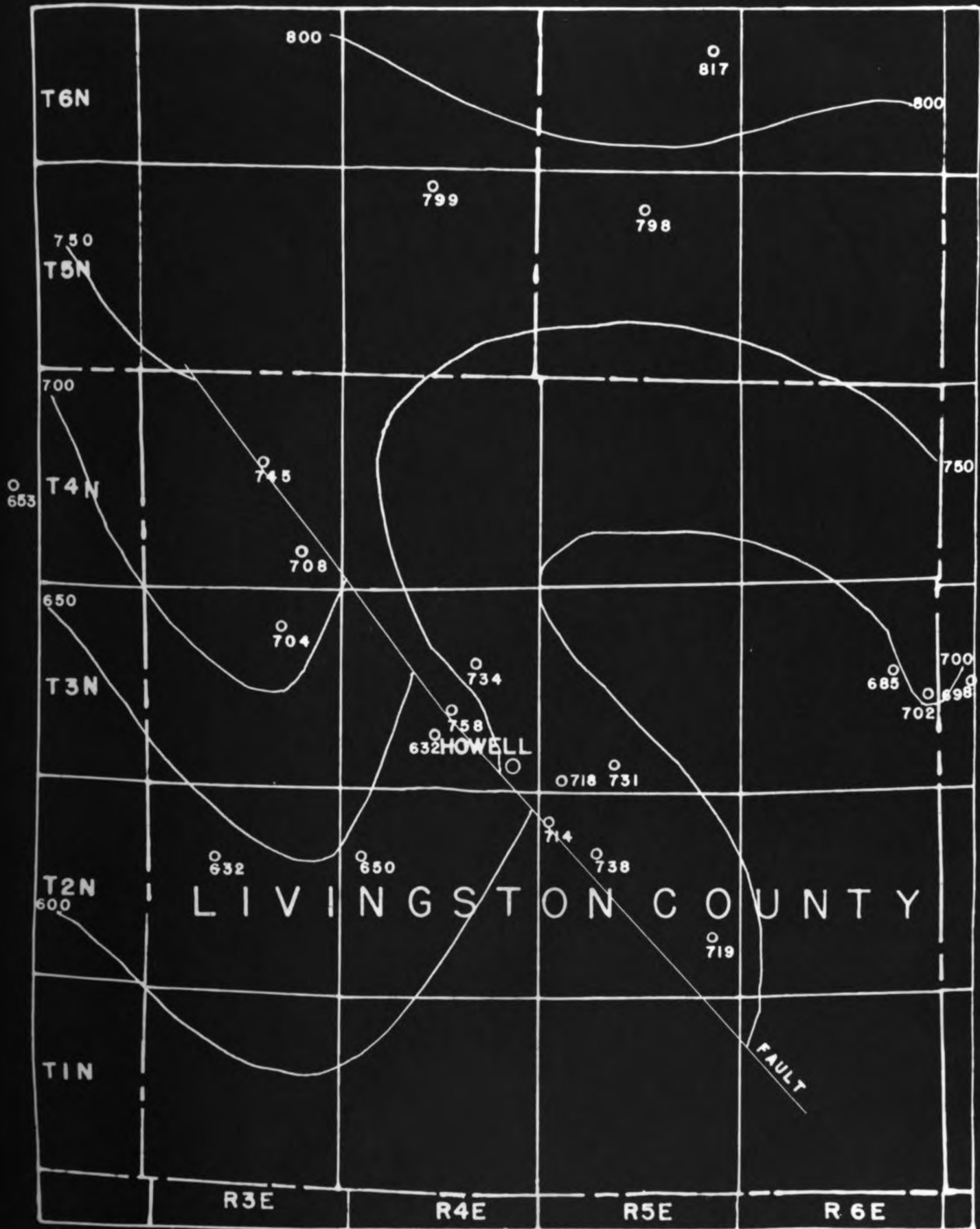
FIGURE 9A ISOPACHOUS MAP SHOWING THE INTERVAL BETWEEN THE BASE OF THE SUNBURY SHALE AND THE TOP OF THE DUNDEE LIMESTONE ISOPACHOUS INTERVAL 50 FEET
