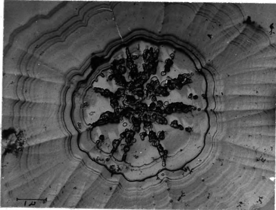
Figure 15. Micrograph of an etch pit made by deteriorated Bright Dip. Magnification 14,000 X.
