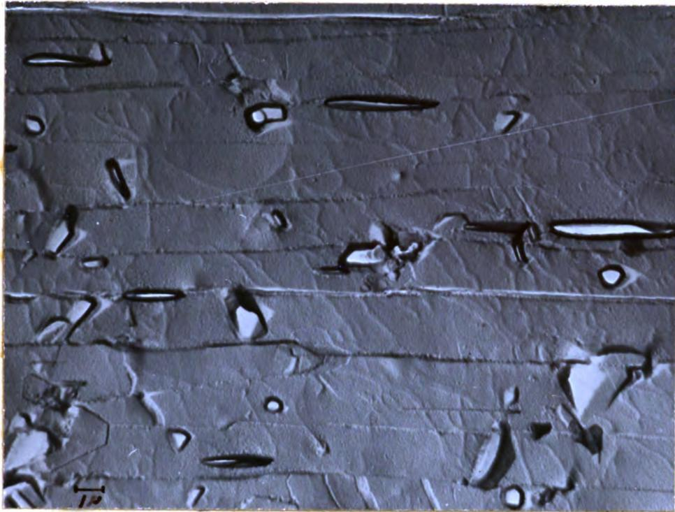
Figure 18. Micrograph illustrating the orientation of silicon precipitates with respect to slip lines. Magnification 4500 X.
