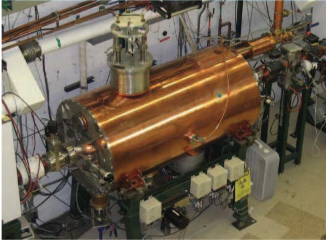
Figure 3.4: Photograph of the RF-kicker, installed in the S1/S2 vaults. The vacuum vessel is a cylindre made of copper-plated steel with an inner diameter of 0.9 m. The beam enters the cavity from the left. The end of the RF guide connected to the RF coupler is visible at the top right. Figure reproduced from [55].
