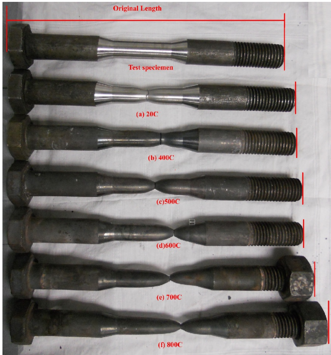
Figure 4.24 – Illustration of fracture surfaces in A490 bolts at various temperatures
