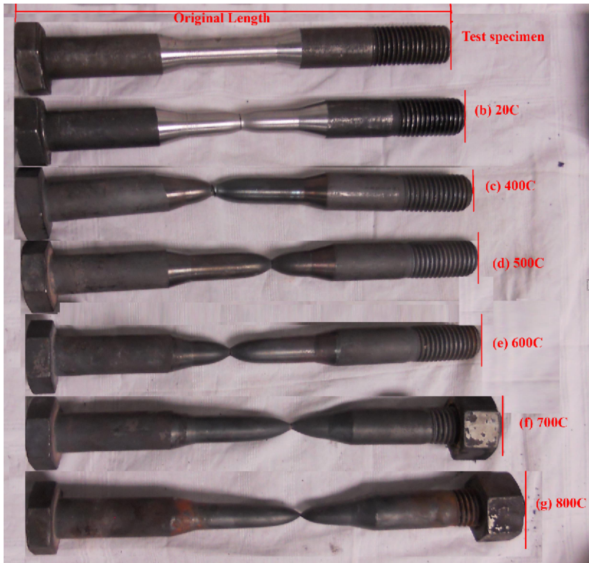
Figure 4.22 – Illustration of fracture in A325 bolts at various test temperature fractured test specimen after test
