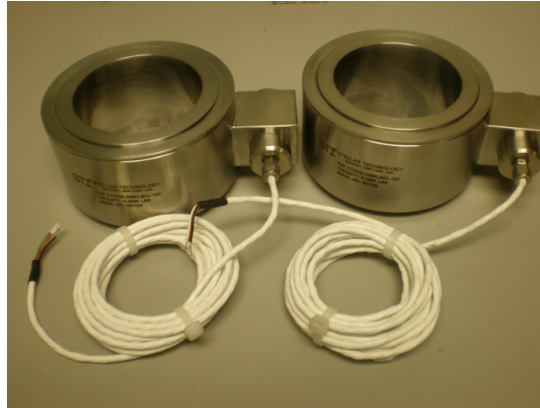
Figure 4.7 – Donut shaped load cells to record load during the mechanical tests
