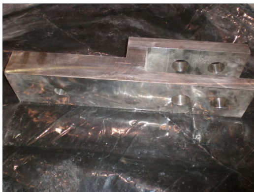
(c) Y-shaped shear anchorage plate to perform shear test
