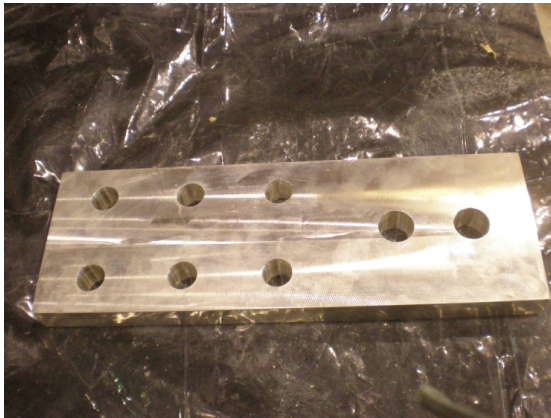
(a) Anchorage plate connected to the loading frame to facilitate the connection for shear and tension anchorage plates
