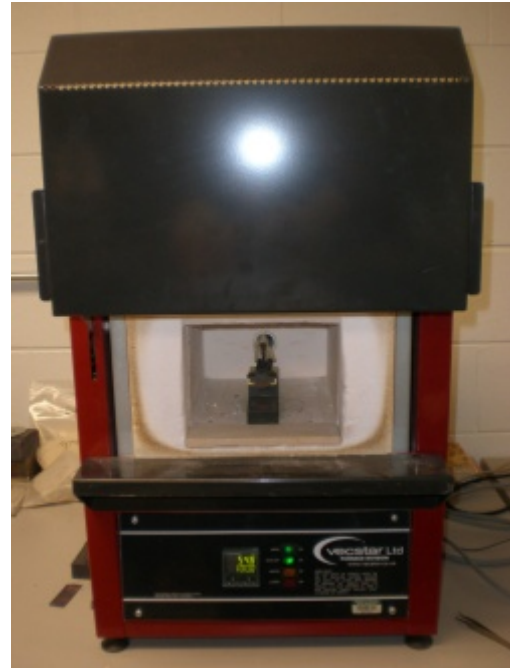
(c) Electric furnace for high temperature tests
