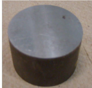
Figure 3.1 – Typical test specimen for undertaking thermal conductivity and specific heat tests
