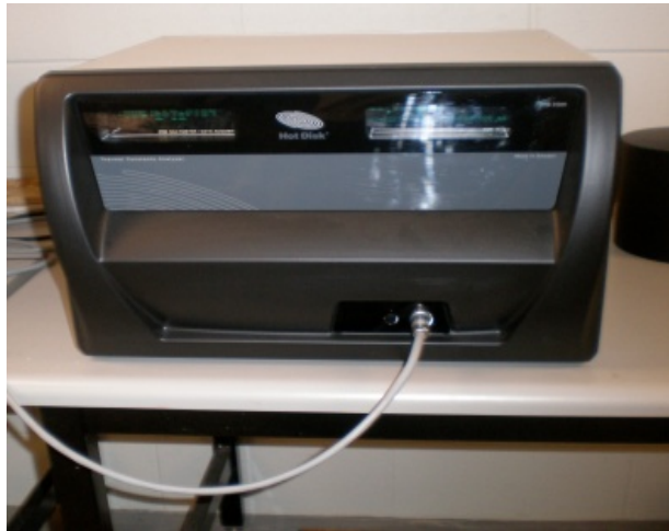
(a) Hot Disk (TPS 2500) thermal constant analyzer
