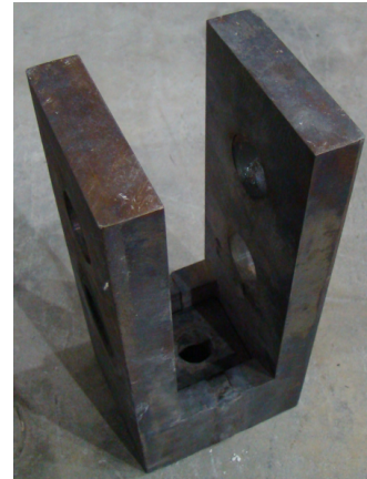
(b) Tension anchorage plate to perform tension test
