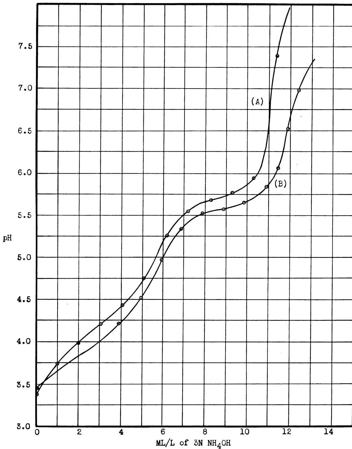
Fig. 1. Potentiometric titration of plating solutions. Solution(A) 3.4 g./l. of \text{FeSO}_4 \cdot 4\text{H}_2\text{O} . Solution (B) 3.4 g./l. of \text{FeSO}_4 \cdot 4\text{H}_2\text{O} , 5.0 g./l. of \text{H}_3\text{BO}_3 .
