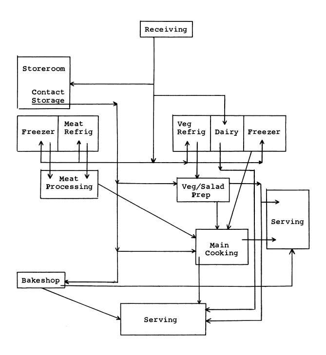
Figure 10. Incoming flow and distance relationship chart: the proposed layout.
