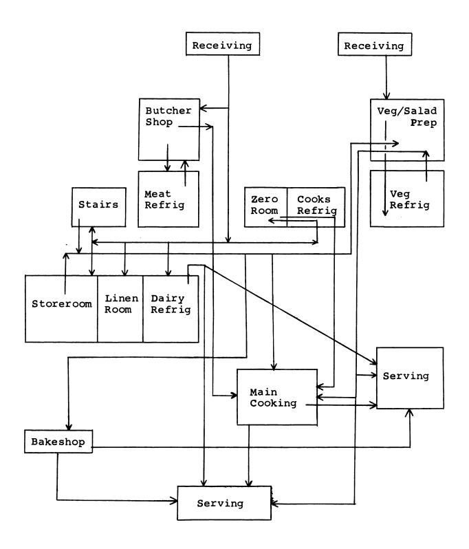
Figure 9. Incoming flow and distance relationship chart: the original layout.
