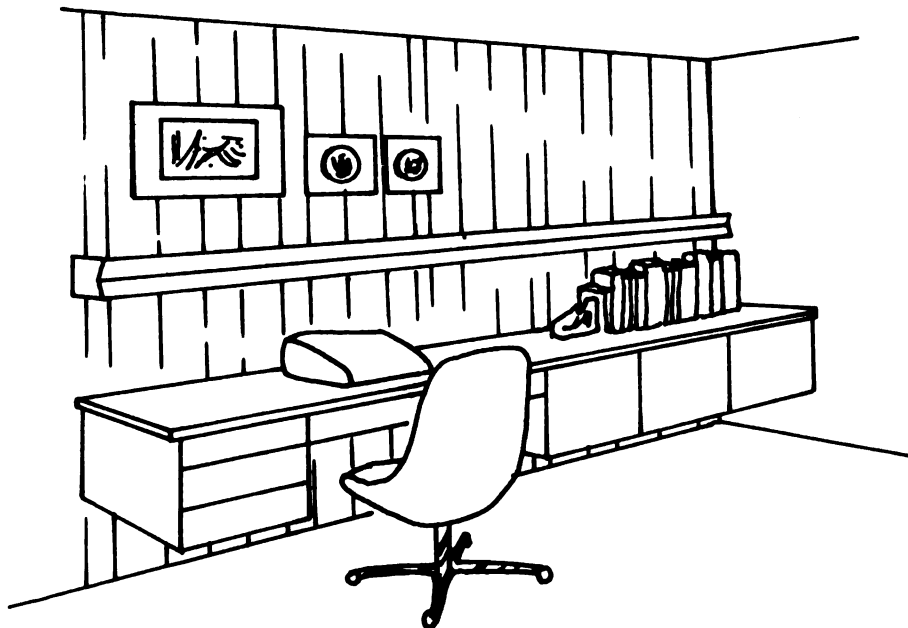
4. Low Wall Bracket Lighting
