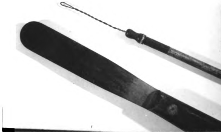
Figure 1. A coiled nickel-chromium alloy wire was used to penetrate and sample the selected organ and tissue sites. The spatula was used to sear tissue surfaces before sampling.
