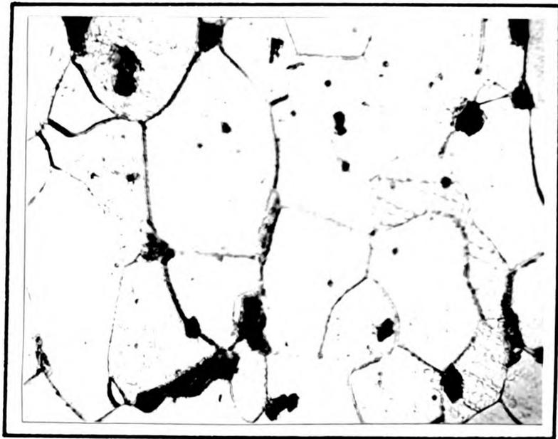
As the low-carbon steel, XX' cools, individual ferrite grains or a solid solution of alpha iron plus carbon crystallizes. If any of these ferrite grains contain less than .06% carbon, then at the point A, cementite is precipitated out.
