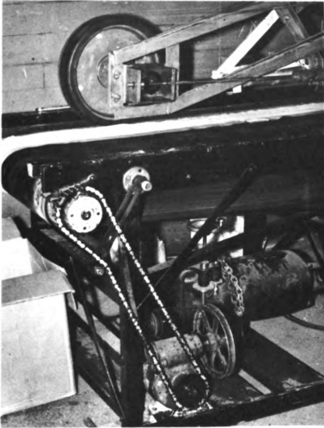
Fig. 26 - Moving belt power system and how it is transmitted to the planter's powered system.
