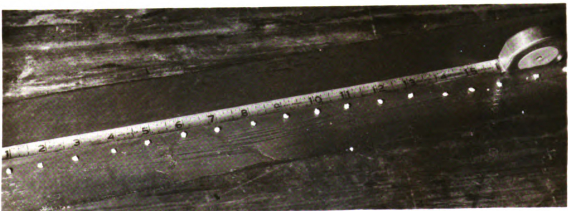
Fig. 9 - Seeds planted with the plastic model. Scale provides a comparison means to show its accuracy.
