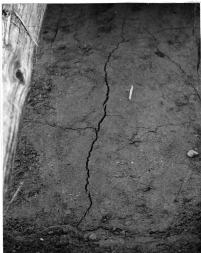
Figure 11. Ground failure caused by circular anchor.
