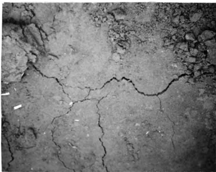
Figure 12. Ground failure caused by square anchor.
