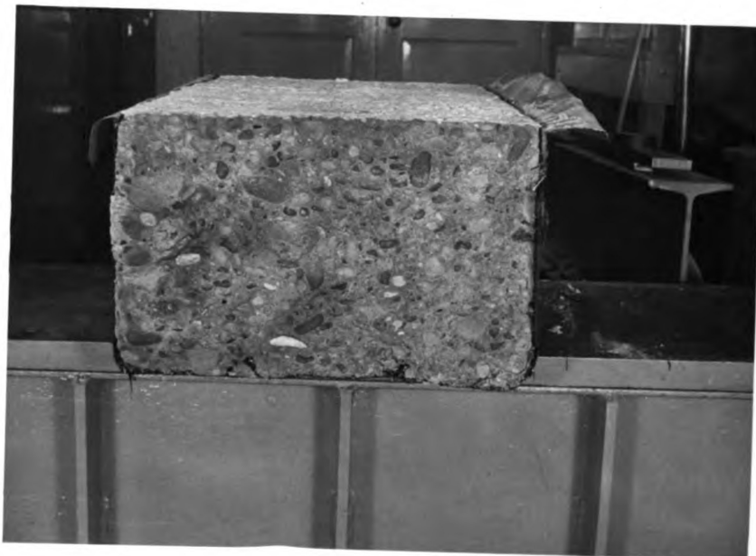
9. Section of beam cured seven days with wet burlap followed by three days of no curing on waterproof subgrade. Dehydrated layer is thin, well defined and about 1/16 " thick.
