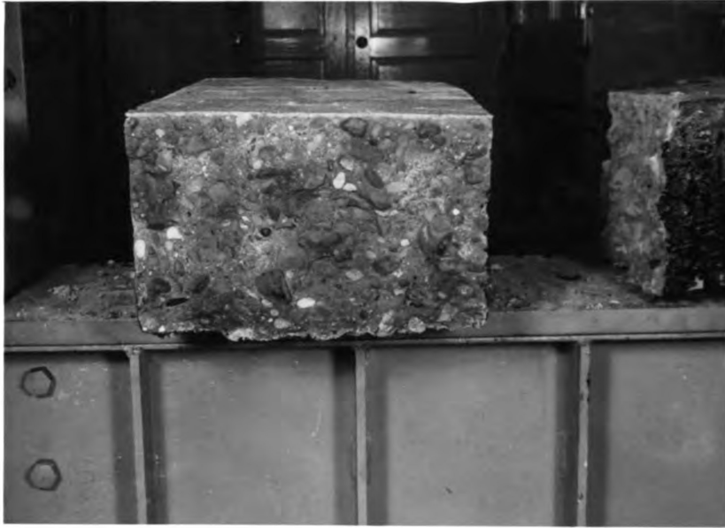
11. Section of beam cured with clear membrane, on dry sand subgrade. Dehydration line is sharply defined and about 1/8 " thick.
