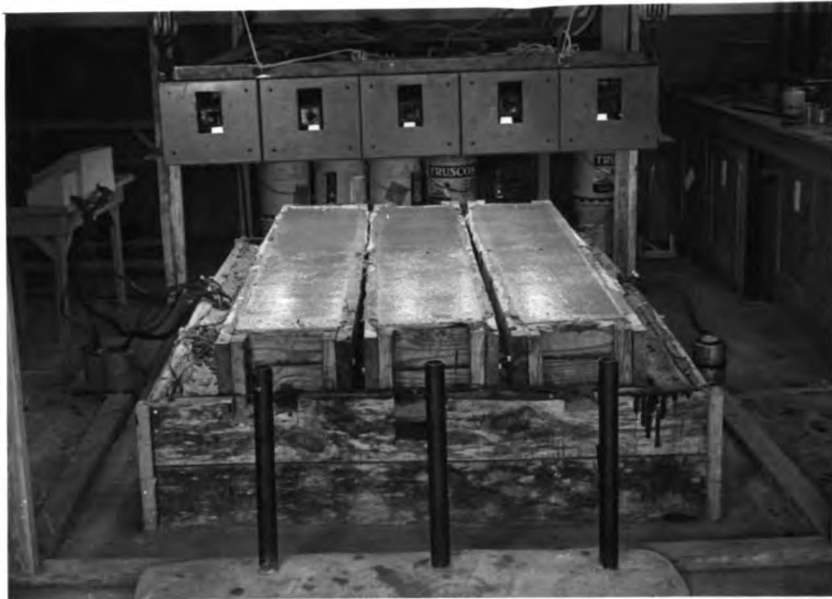
7. End posts used as reference for length change are located in center foreground. Plugs for warping measurements are faintly visible on beam surfaces.
