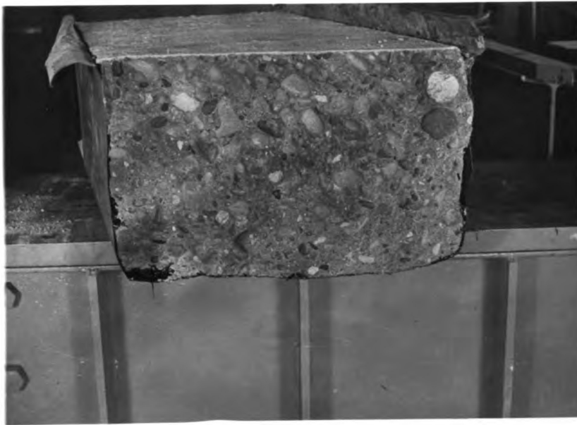
9. Section of beam cured seven days with wet burlap followed by three days of no curing on waterproof subgrade. Dehydrated layer is thin, well defined and about 1/16 " thick.
