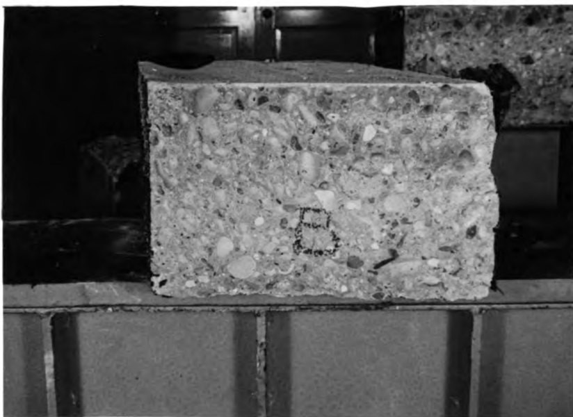
14. Section of beam with no curing on wet sand subgrade. Dehydration line is sharply defined and about 3/16 " thick.
