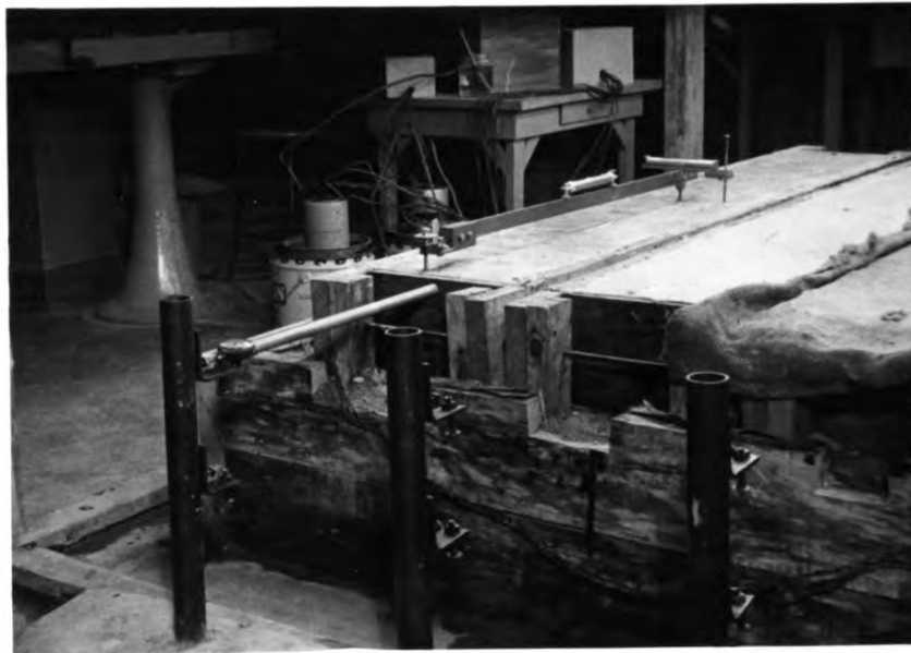
6. The clinometer for warping measurements is shown at right center. The length change reference rod is shown at left center.
