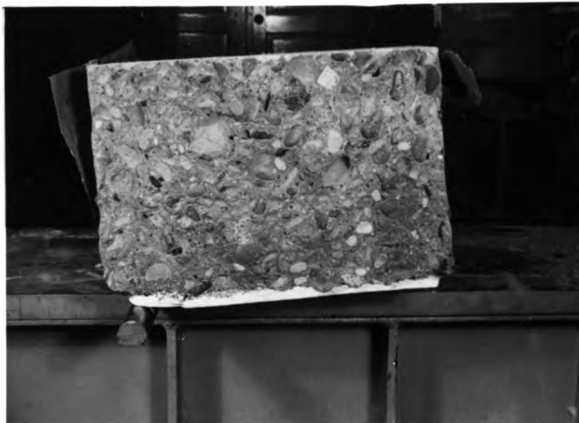
12. Section of beam cured seven days with wet burlap followed by three days of no curing on dry sand subgrade. Dehydration line is sharply defined and about 1/16 " deep.
