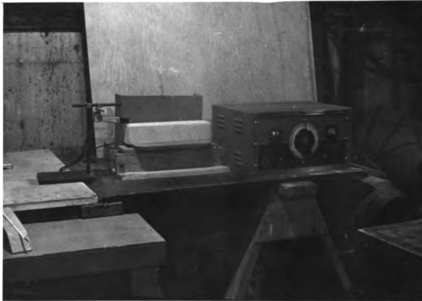
3. Sonic apparatus for determining dynamic modulus of elasticity.
