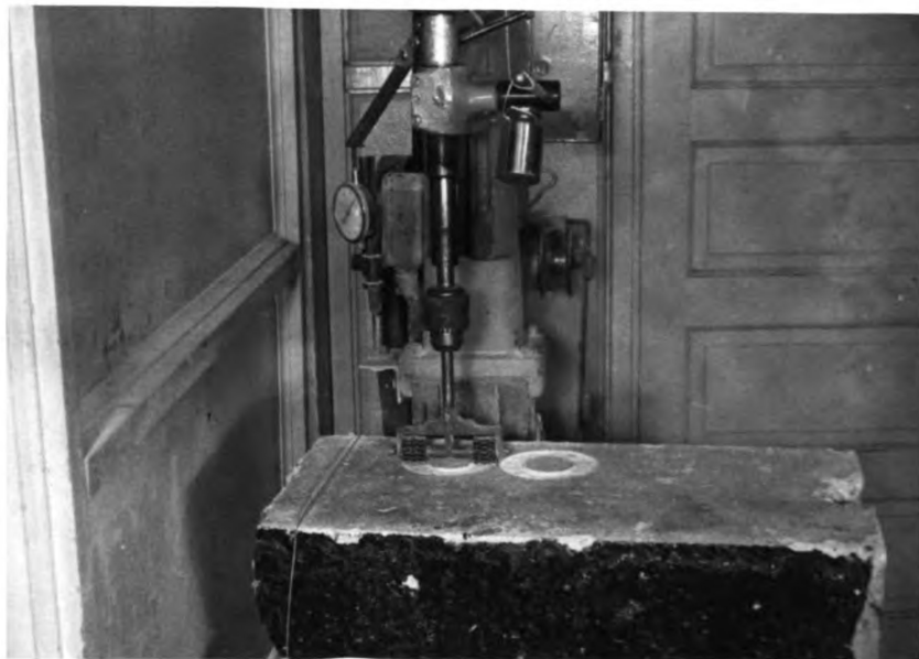
16. Beam end subjected to wear test. Dial for measuring penetration is visible at left center.
