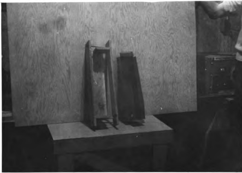
1. Mold Assembly; waterproof paper liner is shown on the right.
