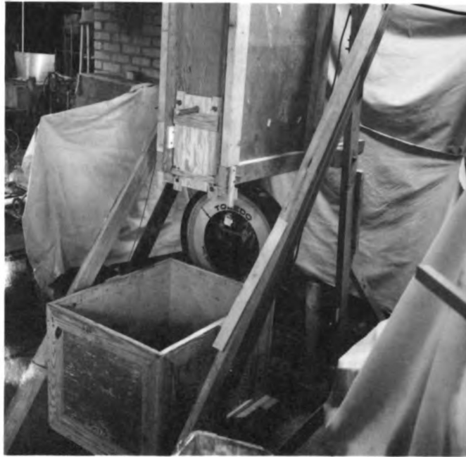
Fig. 1 - An overall view of the apparatus showing the stationary hopper above the movable bin.
