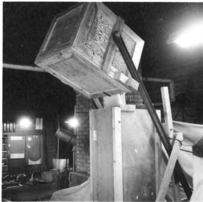
Fig. 2 - The movable bin in position to dump the corn into the hopper.
