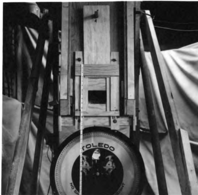
Fig. 6 - The equipment in position prior to taking measurements on the flow of corn through a vertical opening.
