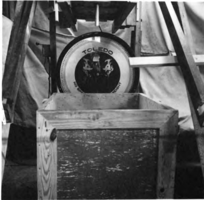
Fig. 5 - The equipment in position prior to taking measurements on the flow of corn through a horizontal opening.
