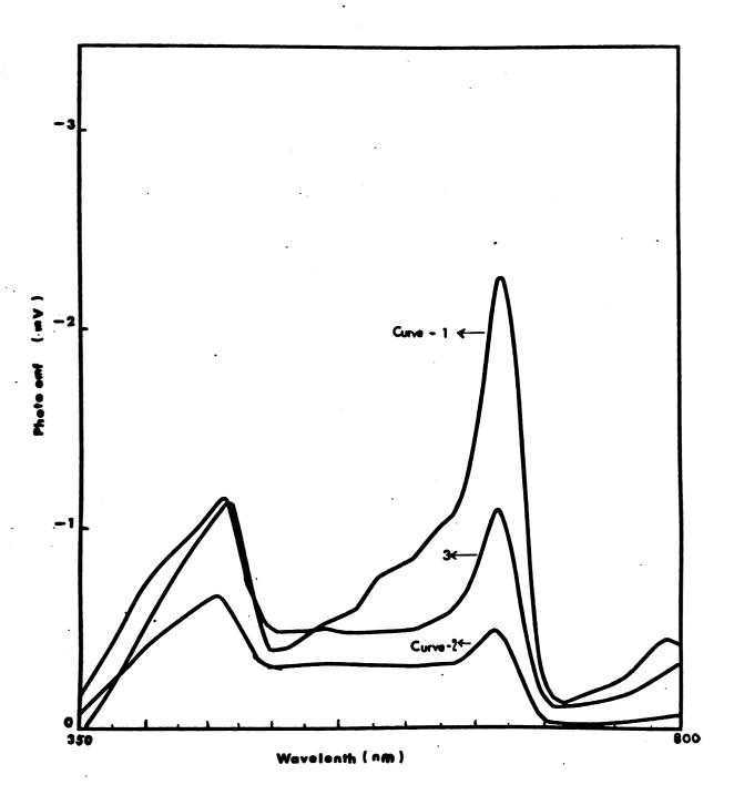
recorded from a single membrane. Spectrum 2 in Figure 26 was taken after one hour of alternative illumination at 670 nm and 440 nm.
